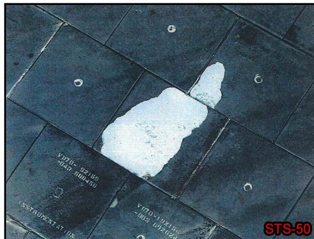
Figure 4.4.5.2b Detailed view of wing tile damage, STS-50
