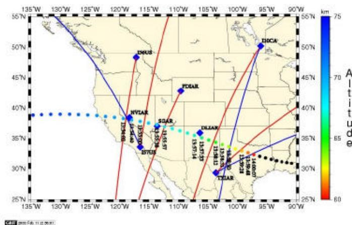
Figure 8-1: Projected track, altitude, time GMT, and infrasonic detections for the Columbia reentry based on using PMCC with time windows greater than 30 s. (The red lines indicate the observed azimuth of the first arrival, and the blue lines the azimuth of any secondary arrivals.) [18]
