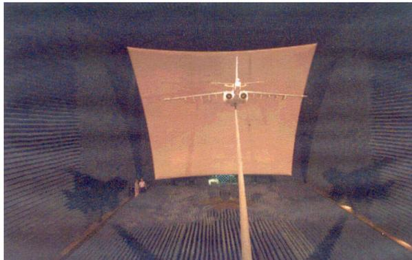
Figure 8 – The AFRL Advanced Compact RCS Measurement Range (ACR)
