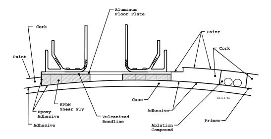
Figure 1. TPS Adjacent to Sytems Tunnel Floor Plate
