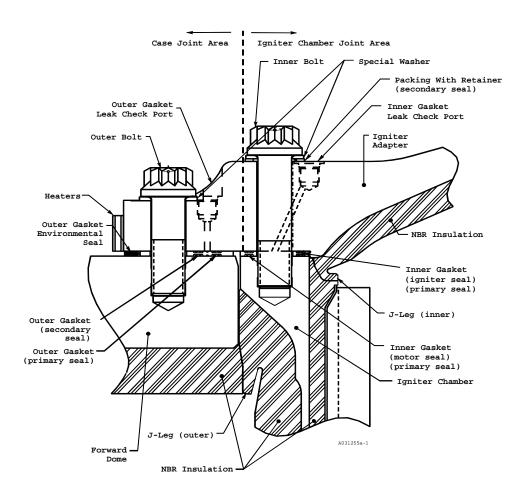
Figure 1. Igniter Adapter-to-Chamber Joint and Igniter Adapter-to-Case Joint
