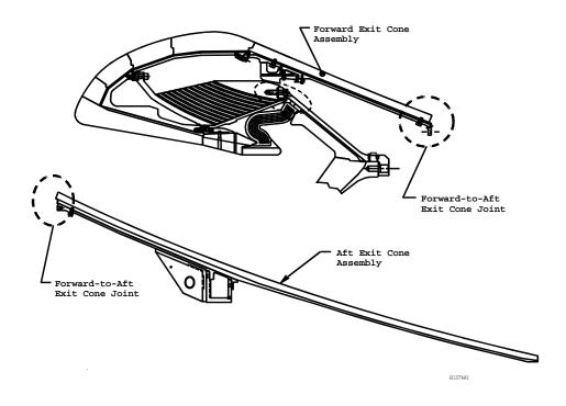
Figure 1. Forward-to-Aft Exit Cone Joint Location
