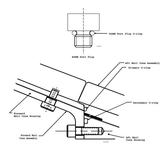
Figure 2. Forward-to-Aft Exit Cone Joint O-ring and Leak Check Port
