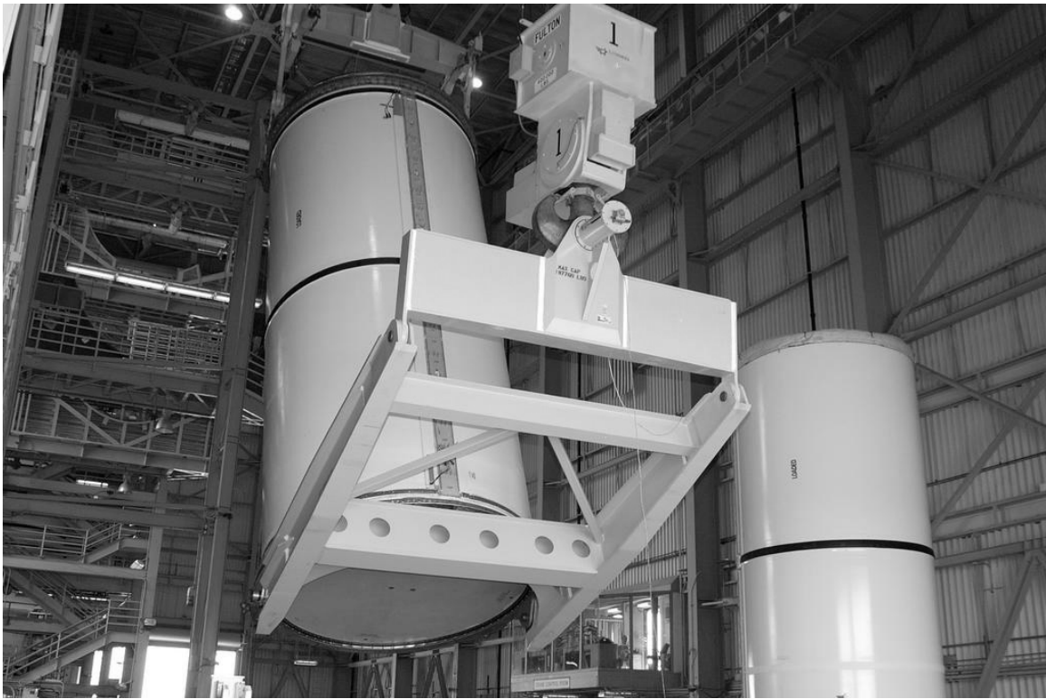
Figure No. E-41. SRB segment being lifted and rotated, 2004. Source: NASA John F. Kennedy Space Center, KSC-04PD-0058, accessed at http://mediaarchive.ksc.nasa.gov/search.cfm .
