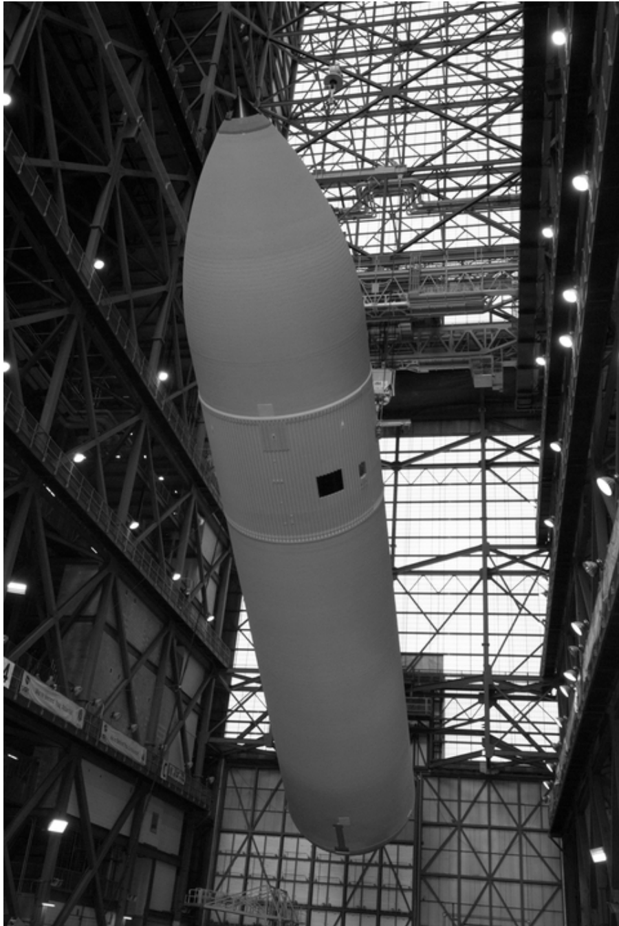
Figure D-41. ET-135 being rotated to vertical in KSC's VAB for placement into a test cell, January 6, 2010.
