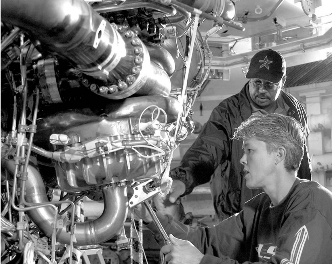
Figure C-10. Final preparations being made to a SSME for testing, direction unknown, October 25, 2005.
