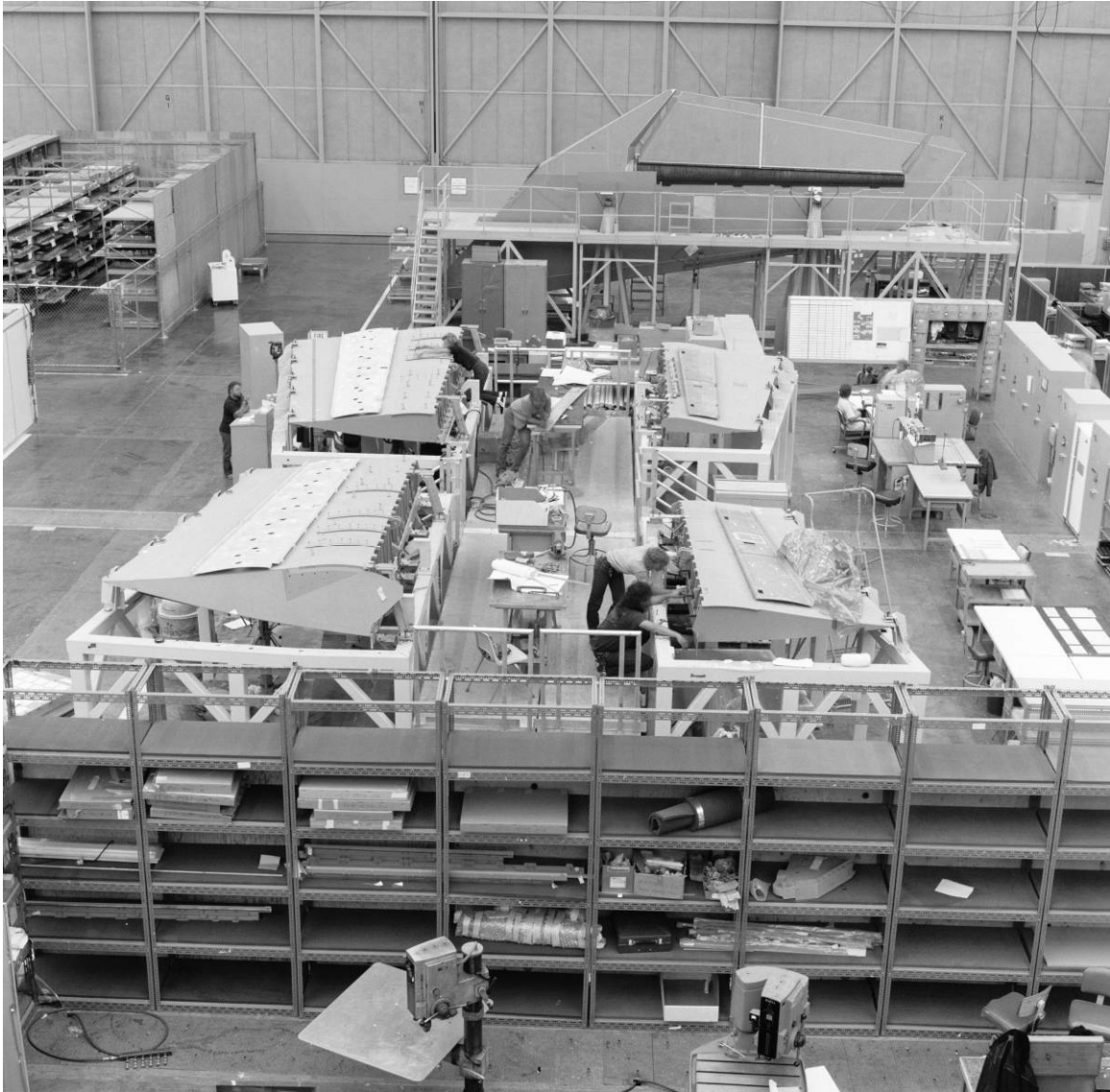
Figure B-27. Inspection of Discovery's elevons, High Bay 1, AFP 42, September 14, 1982.
