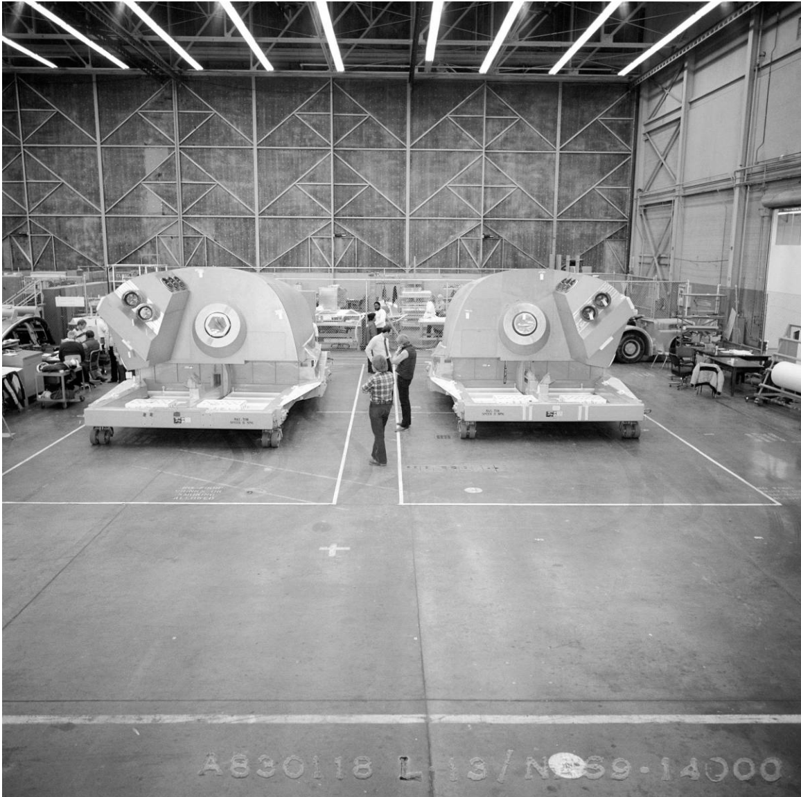
Figure B-38. Discovery's two OMS pods upon arrival at AFP 42, January 18, 1983. Source: NASA, Johnson Space Center Image Repository, JSC2010-03408.
