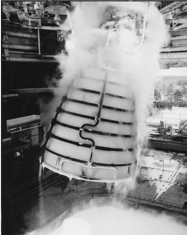
Figure C-17. A Block I SSME undergoing testing on Stand A-1, direction unknown, 1995. Source: John C. Stennis Space Center, SIRS, 95-088-1, accessed at http://www.ssc.nasa.gov/sirs/scripts/xmlWelcome.pl .
