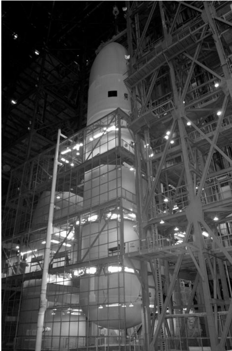
Figure D-42. The ET for STS-114 being lifted from a test cell in KSC's VAB for mating, February 28, 2005.
