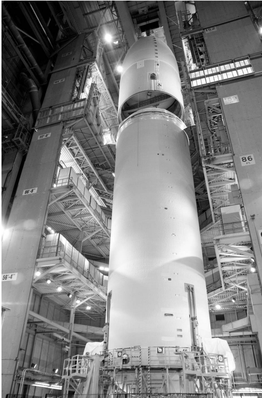
Figure D-34. LO2/intertank combination being moved to Cell A at MAF for stacking on top of the LH2 tank to complete ET-133, February 4, 2009.
