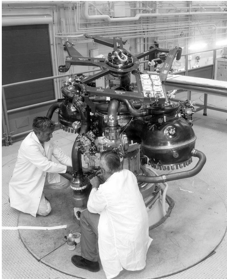
Figure C-30. Rocketdyne technicians connect a Powerhead Duct to a Combustion Device on SSME 0004, 1976.
