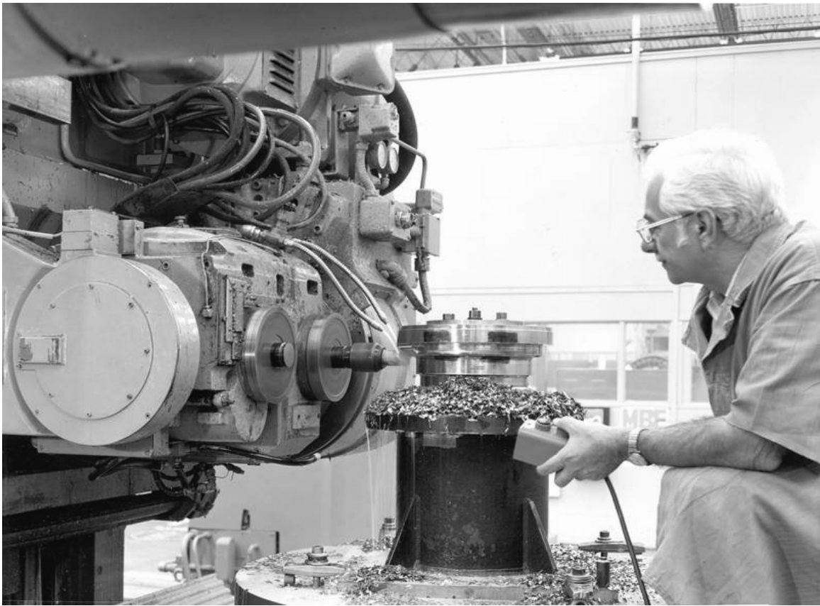
Figure C-26. A technician machining a SSME Oxidizer Preburner Body on the 5-Axis Omni Mill, Canoga Park, 1973.
