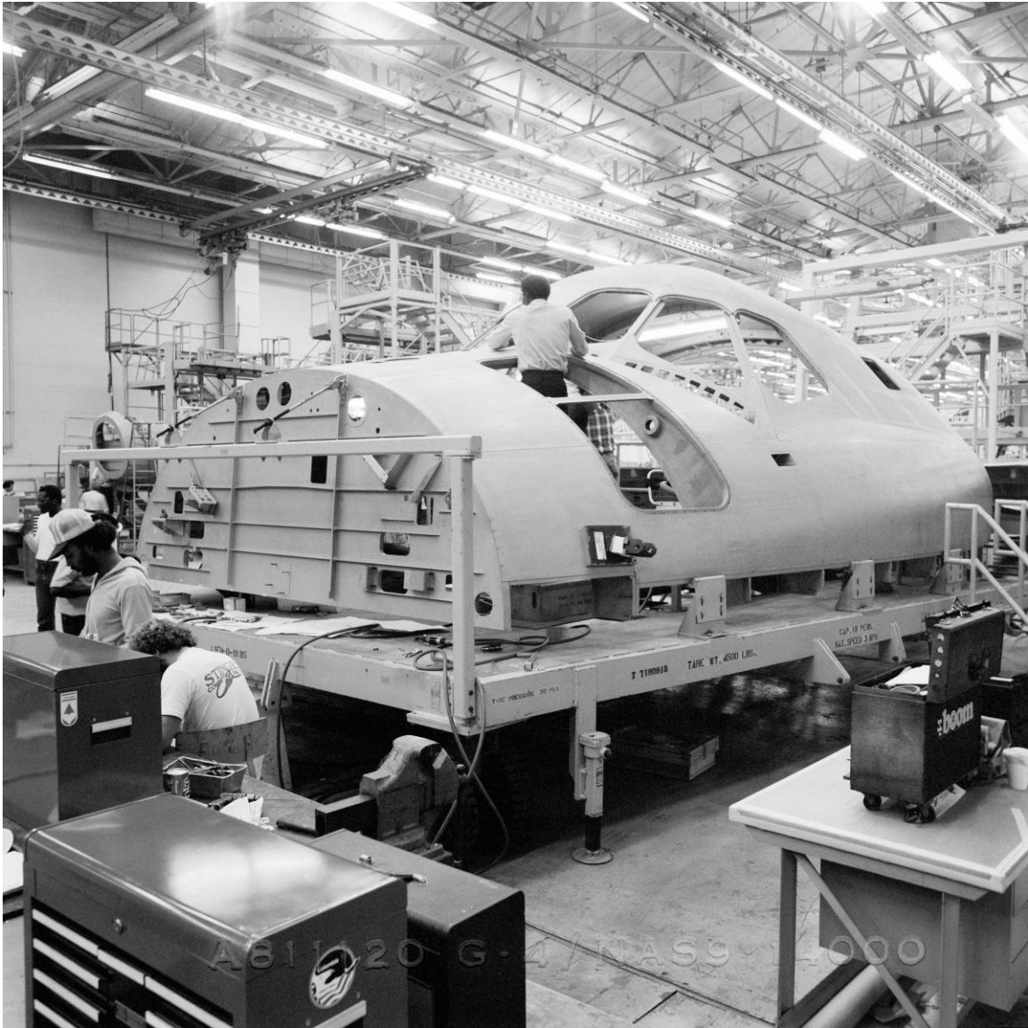
Figure B-4. Manufacturing of Discovery's upper forward fuselage, NAR Building 290, Downey, California, November 20, 1981. Source: NASA, Johnson Space Center Image Repository, JSC2010-03204.
