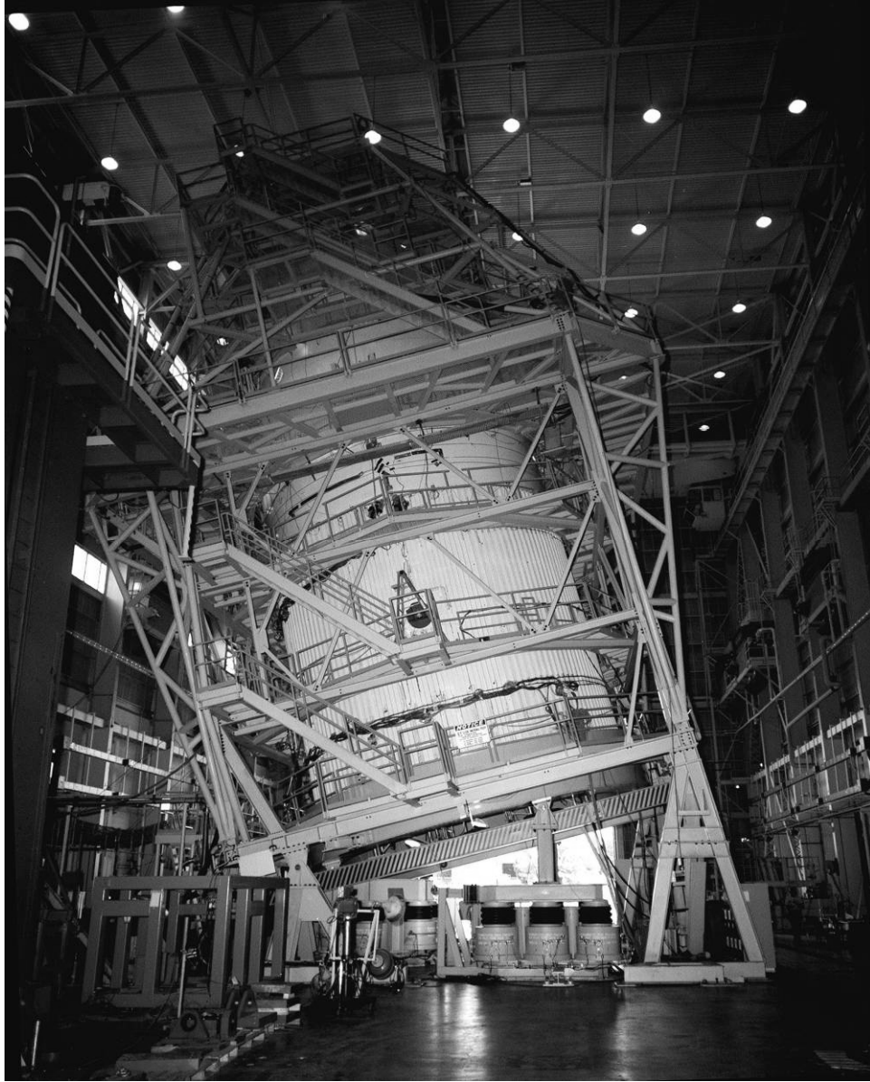
Figure D-2. Liquid oxygen tank of the ET during a hydroelastic modal test at MSFC, May 1, 1978.
