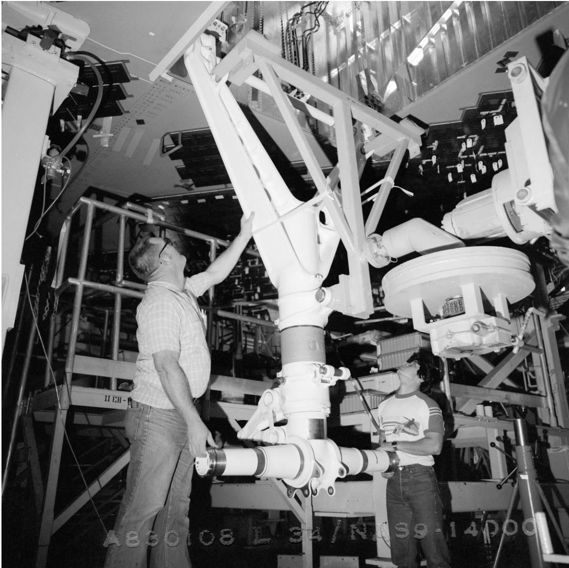
Figure B-35. Installation of Discovery's port side main landing gear in High Bay 2, AFP 42, January 8, 1983. Source: NASA, Johnson Space Center Image Repository, JSC2010-03396.
