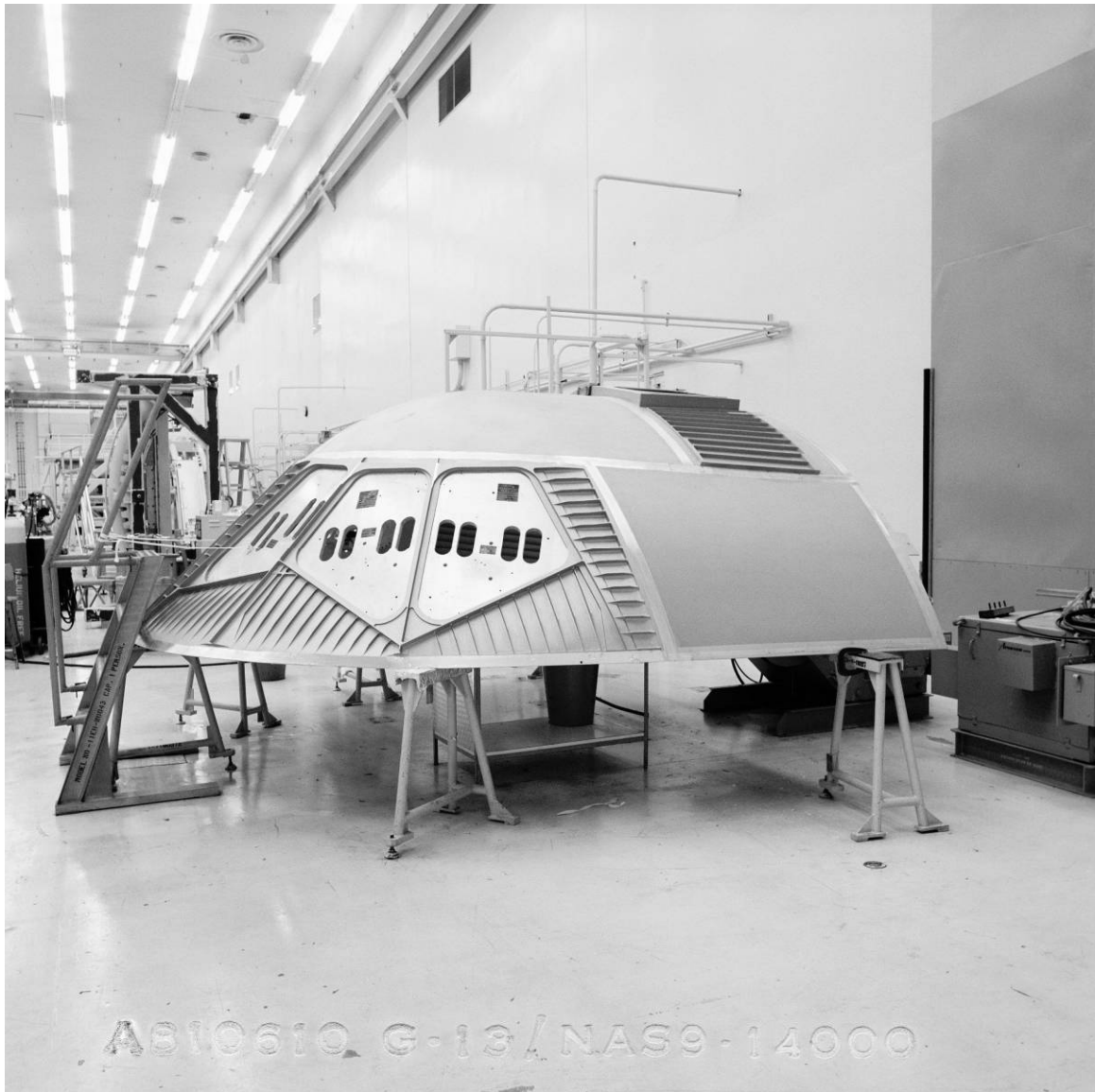
Figure B-6. Upper skin panel assembly for Discovery's crew module, NAR Building 290, Downey, California, June 10, 1981. Source: NASA, Johnson Space Center Image Repository, JSC2010-03105.
