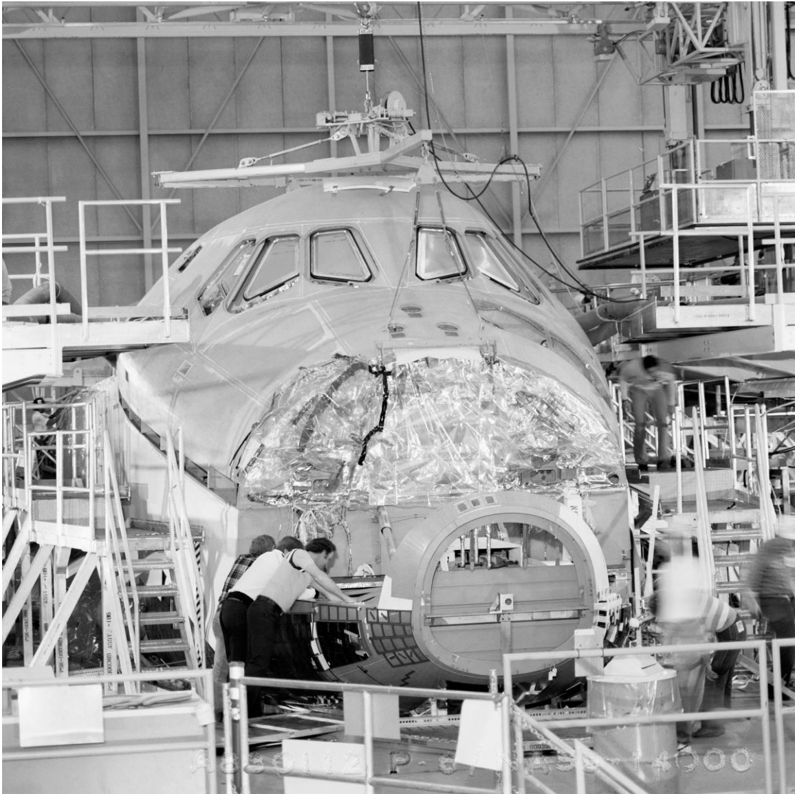
Figure B-37. Installation of Discovery's upper forward fuselage in High Bay 2, AFP 42, January 12, 1983.
