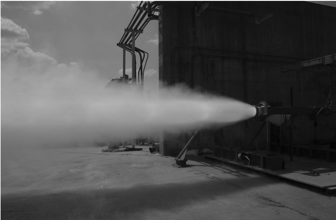
Figure No. E-10. Space Shuttle SRB separation motor test firing at Test Stand 116 at MSFC, March 28, 2007.
