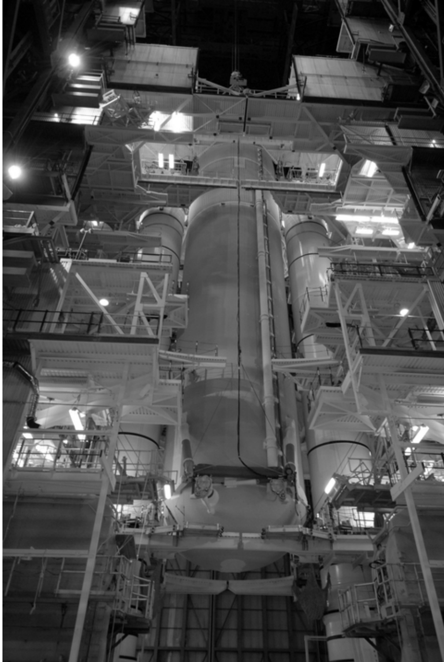
Figure D-43. ET-29 being lowered between the SRBs in KSC's VAB for mating, August 28, 2008.
