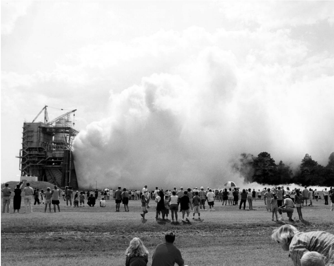
Figure C-18. A Block II SSME undergoing flight certification testing on Stand A-2, camera facing west, July 25, 2000.
