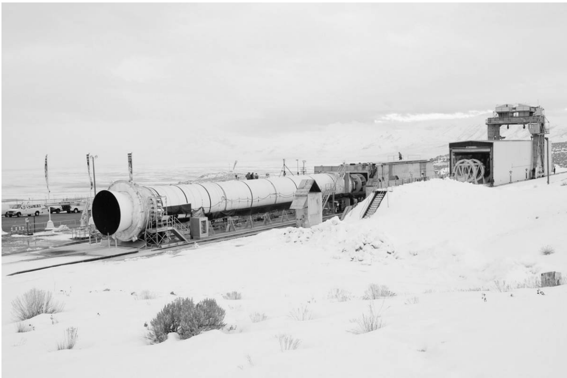
Figure No. E-4. Flight Support Motor (FSM)-17 test, February 25, 2010, at ATK in Promontory, Utah. This was the last RSRM test of the Space Shuttle program. Source: NASA, accessed at http://www.nasa.gov/images/content/429987main_179307_002.jpg .
