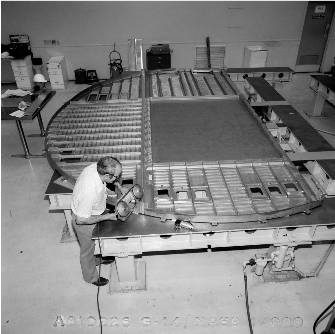
Figure B-5. Manufacturing of Discovery's crew module aft bulkhead, NAR Building 290, Downey, California, February 26, 1981. Source: NASA, Johnson Space Center Image Repository, JSC2010-03081.
