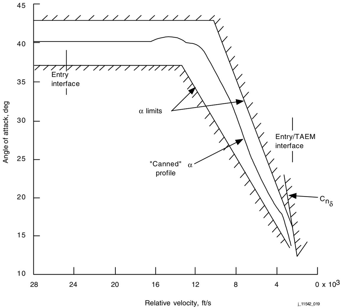
**Figure 5-24. Entry angle-of-attack profile**
