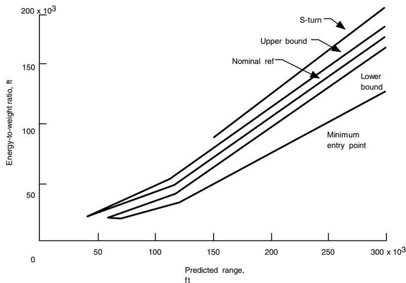
**Figure 2-4. Typical TAEM energy-to-weight ratio**
