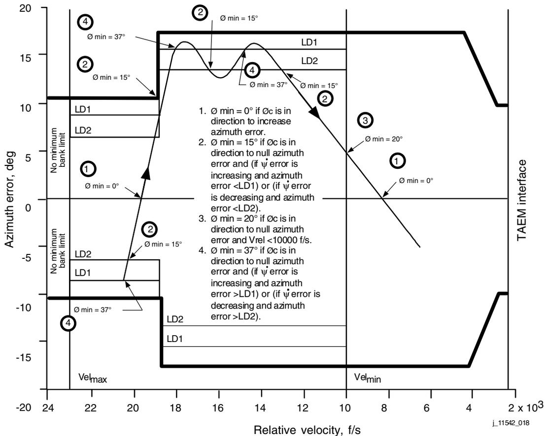
**Figure 5-23. Azimuth error versus relative velocity plot**
