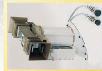
EO-1 HIGH VOLTAGE POWER CONDITIONER
