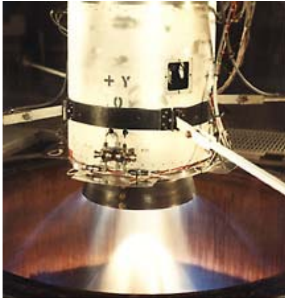
Rocket Engine Firing Inside Vacuum Test Cell
