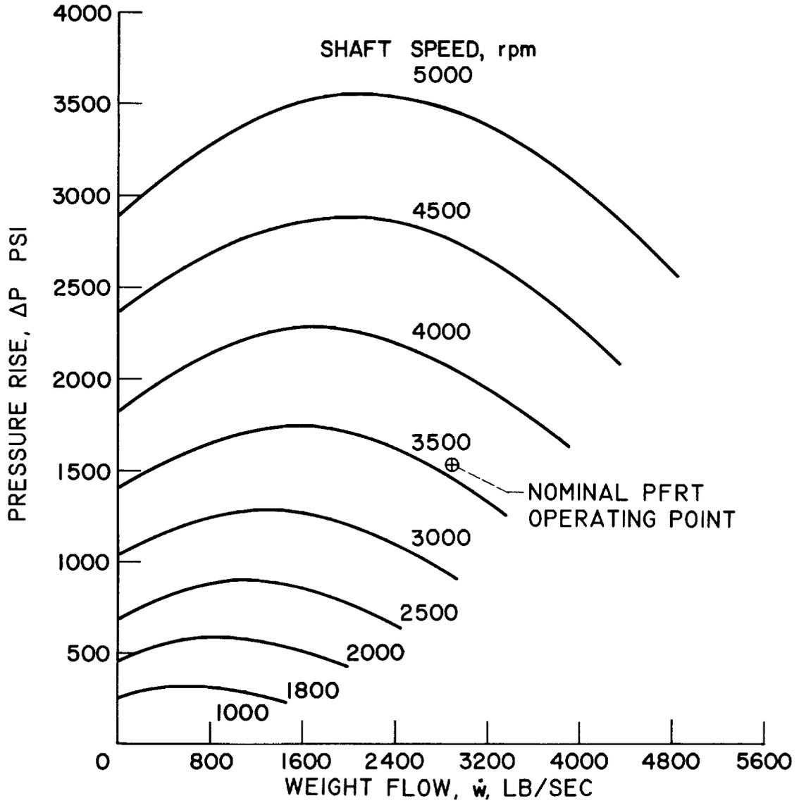
Figure 11. - M-1 Rocket Engine Project - Predicted Oxidizer Pump Performance.
