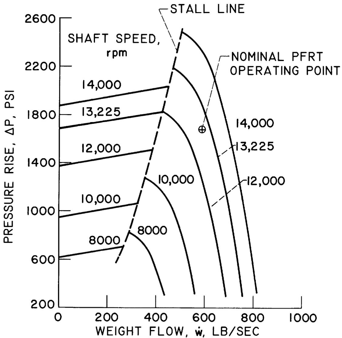
Figure 9. - M-1 Rocket Engine Project - Predicted Fuel Pump Performance.
