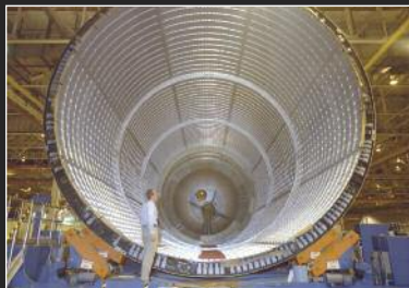
Liquid hydrogen tank showing slosh and vortex baffle inside.
