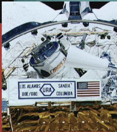
STS-39’s Air Force Program-675 equipment mounted on the experiment support system pallet in Discovery’s payload bay.
