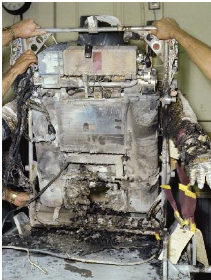
The original shuttle extravehicular mobility unit with an aluminum secondary oxygen pack isolation valve and first-stage regulator ignited and burned during acceptance ground testing on an unoccupied unit in 1980 (left). The redesigned unit with a nickel-copper alloy secondary oxygen pack isolation valve and first-stage regulator is being used with much success (right).
