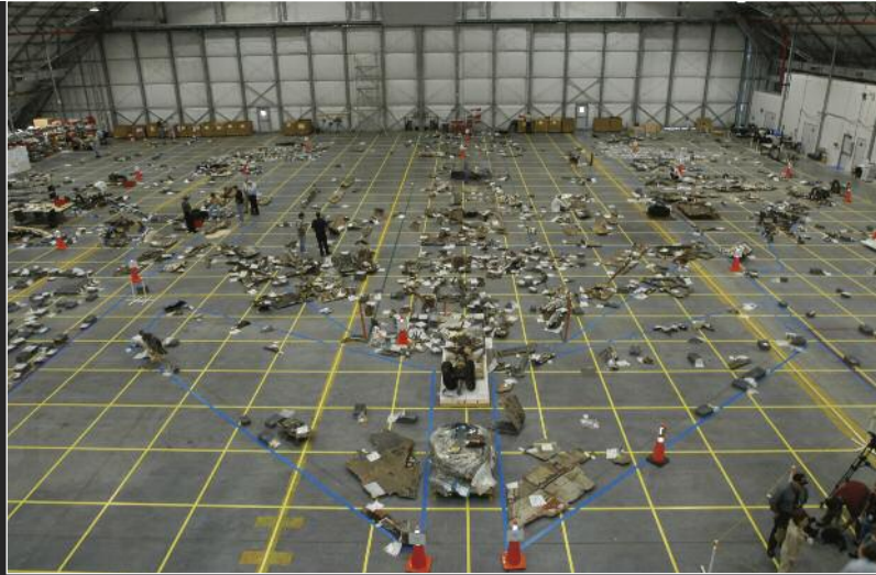
Reconstruction of the Columbia from parts found in East Texas. From this layout, NASA was able to determine that a large hole occurred in the leading edge of the wing and identify the burn patterns that eventually led to the destruction of the shuttle.
