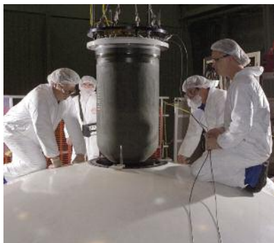
Technicians shown installing igniter used to initiate the propellant burn in a forward motor segment. The igniter was a small rocket motor loaded with propellant that propagated flame down the bore of the motor.
