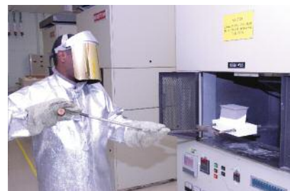
At the Kennedy Space Center tile shop, a worker places a Boeing replacement insulation 18 tile in the oven to be baked at 1,200°C (2,200°F) to cure the ceramic coating.
