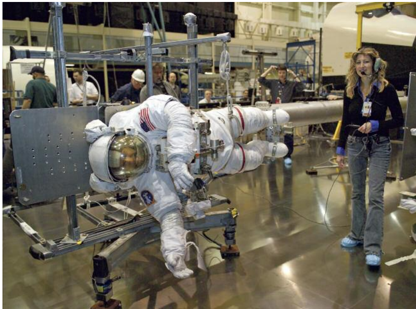
Astronaut Piers Sellers, STS-121 (2006), wearing a training version of the extravehicular mobility unit, participates in an extravehicular activity simulation while anchored on the end of the training version of the Shuttle Robotic Arm in the Space Vehicle Mockup Facility at Johnson Space Center (JSC). The arm has an attached 15-m (50-ft) boom used to reach underneath the Orbiter to access tiles. Lora Bailey (right), manager, JSC Engineering Tile Repair, assisted Sellers.
