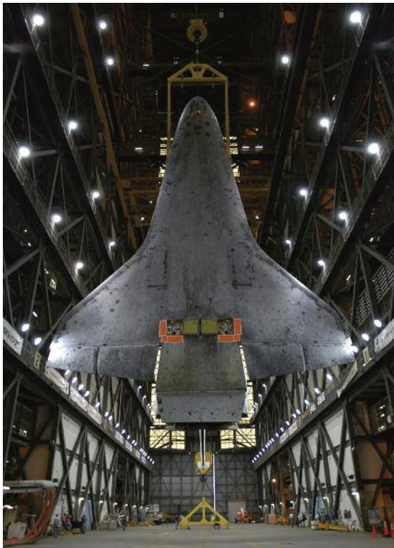
This view of the suspended Orbiter Discovery shows the underside covered with Thermal Protection System tiles.
