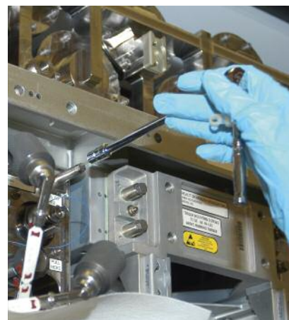
The Microbial Check Valve—measuring 5.1 cm (2 in.) in diameter, 12.7 cm (5 in.) in length—is a stainless-steel cylinder with connections on its ends that facilitated its installation in the shuttle water system line. The cylinder is packed with iodinated ion exchange resin (the base resin is Dowex SBR®). A perforated plate backed by a spring presses against the resin and keeps it compacted to prevent short-circuiting of the water as it flows through the resin.
