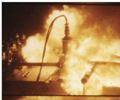
Ignition by particle impact.
