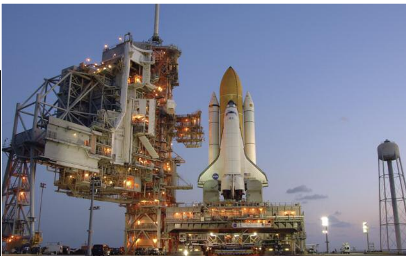
The Space Shuttle arrives at the launch pad, where payloads are installed into the Orbiter cargo bay.
