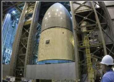
Liquid oxygen tank and intertank in a checkout cell.
