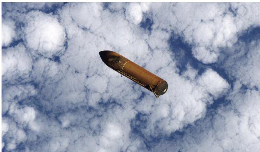
A secondary function of the Thermal Protection System was to stabilize tank internal temperature during re-entry into Earth's atmosphere, thus helping to maintain tank structural integrity prior to its breakup over a remote ocean location.
