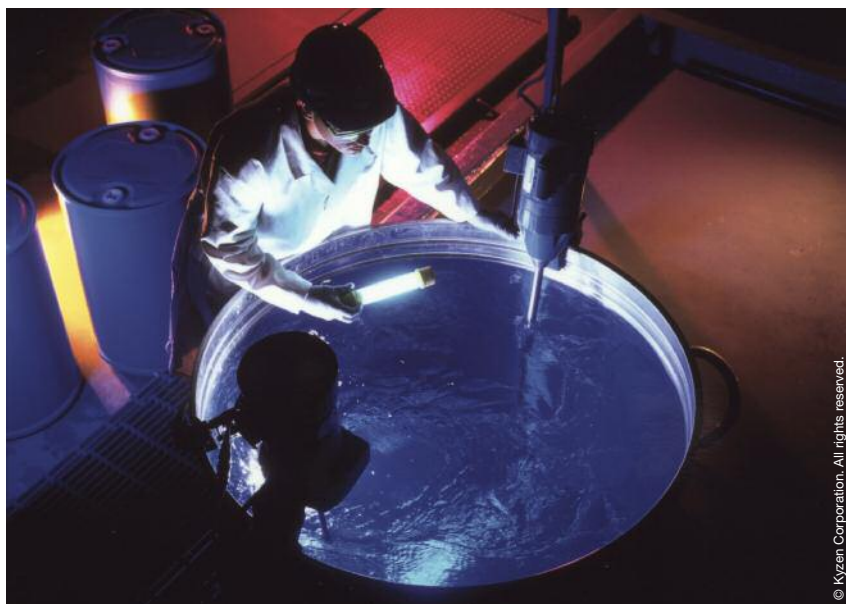
A mixing tank used to produce the cleaning solvent for dissolving solid rocket propellant at Kyzen Corporation. This solvent was free of ozone-depleting chemicals.
