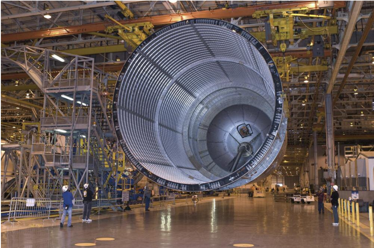
The use of aluminum-lithium Al 2195 in manufacturing major External Tank components, such as the liquid hydrogen tank structure shown above, allowed NASA to reduce the overall weight of the External Tank by 3,402 kg (7,500 pounds). The liquid hydrogen tank measured 8.4 m (27.5 ft) in diameter and 29.4 m (96.6 ft) in length. Photo taken at NASA's Michoud Assembly Facility in New Orleans, Louisiana.
