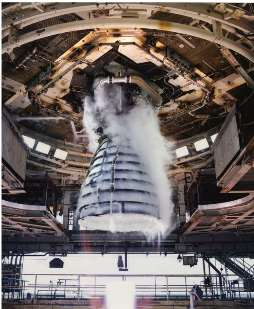
The Space Shuttle Main Engines were the first rocket engines to be reused from one mission to the next. This picture is of Engine 0526, tested on July 7, 2003. A remote camera captures a close-up view of a Space Shuttle Main Engine during a test firing at the John C. Stennis Space Center in Hancock County, Mississippi.
