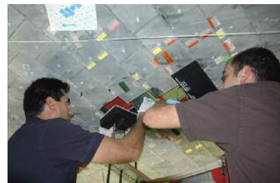
Prior to the launch of STS-119 (2009), Discovery gets boundary layer transition tile, which monitors the heating effects of early re-entry at high Mach numbers.
