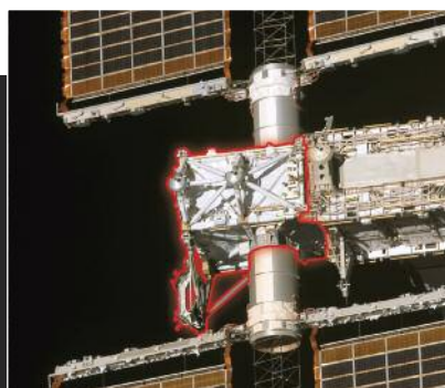
Discovery (STS-116) delivered P5 truss.
