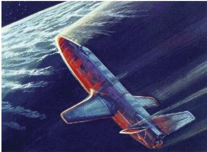
Early conceptual designs for the Orbiter looked much like a traditional airplane with a fairly sharp nose, straight wings, and common horizontal and vertical stabilizers, as shown in this artist's rendering. As a result of subsequent aerodynamic and aerothermodynamic testing and analysis, NASA made the nose more spherical to reduce heating and used a double delta wing planform due to the severe heating encountered by straight wings and the horizontal stabilizer.
