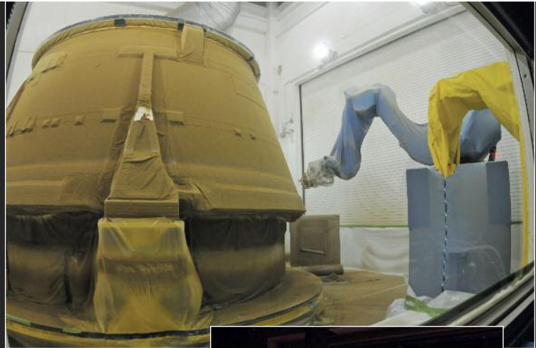
An SRB aft skirt receives a robotically controlled layer of Marshall Convergent Coating-1 Thermal Protection System material.
