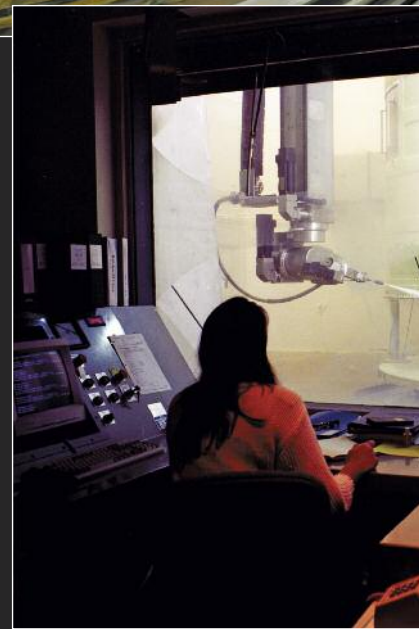
A technician in a control booth monitors the robotic high-pressure hydrolase as it strips Thermal Protection System material from an SRB forward skirt.
