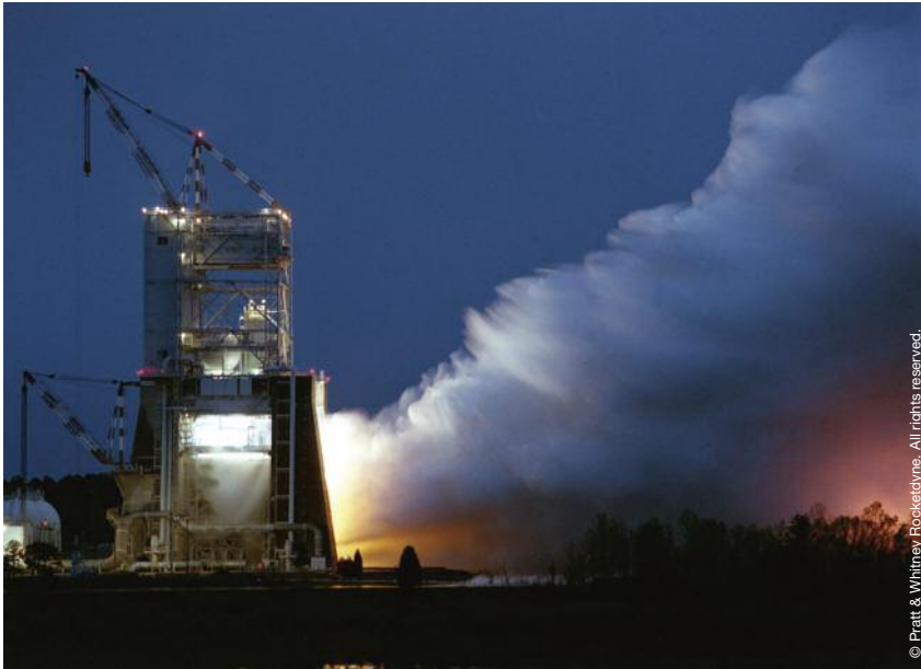
The Technology Test Bed Space Shuttle Main Engine test program was conducted at Marshall Space Flight Center, Alabama, between September 1988 and May 1996. The program demonstrated the ability of the main engine to accommodate a wide variation in safe operating ranges.
