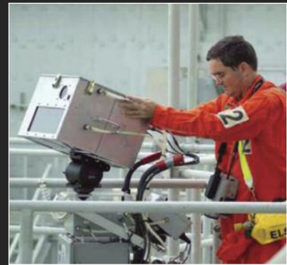
Robert Speece, NASA engineer, is shown operating the ice detection system at the pad, prior to shuttle launch.
