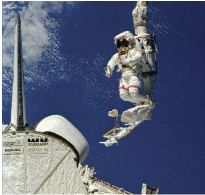
Cherry picking—On STS-41B (1984), Astronaut Bruce McCandless tests a mobile foot restraint attached to the Shuttle Robotic Arm. This device, which allowed a crew member to have a movable platform in space from which tasks could be accomplished, was used by shuttle crews throughout the program.
