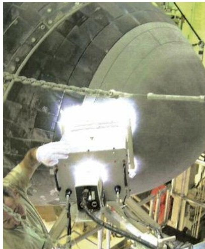
Infrared thermography inspection of the Orbiter nose captured at the instant of the xenon lamp flash. Kennedy Space Center Orbiter Processing Facility.
