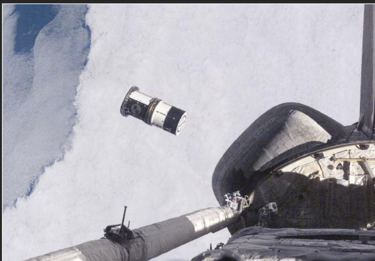
A Department of Defense pico-satellite known as Atmospheric Neutral Density Experiment (ANDE) is released from the STS-116 (2006) payload bay. ANDE consists of two micro-satellites that measure the density and composition of the low-Earth orbit atmosphere while being tracked from the ground. The data are used to better predict the movement of objects in orbit.
