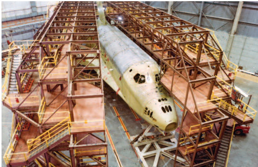
Test rig surrounds the Orbiter structural test article, Challenger, at the Lockheed Test Facility in Palmdale, California.
