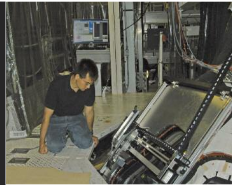
Bradley Burns, lead engineer in the development of the window inspection tool, monitors its progress as it scans an Orbiter window.
