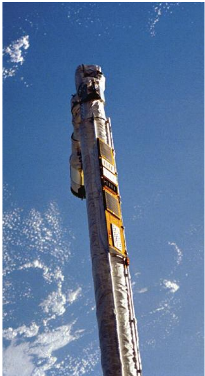
The Intelsat Solar Array Coupon flight experiment shown mounted on the Shuttle Robotic Arm lower arm boom and exposed to space environment conditions during STS-41 (1990).
