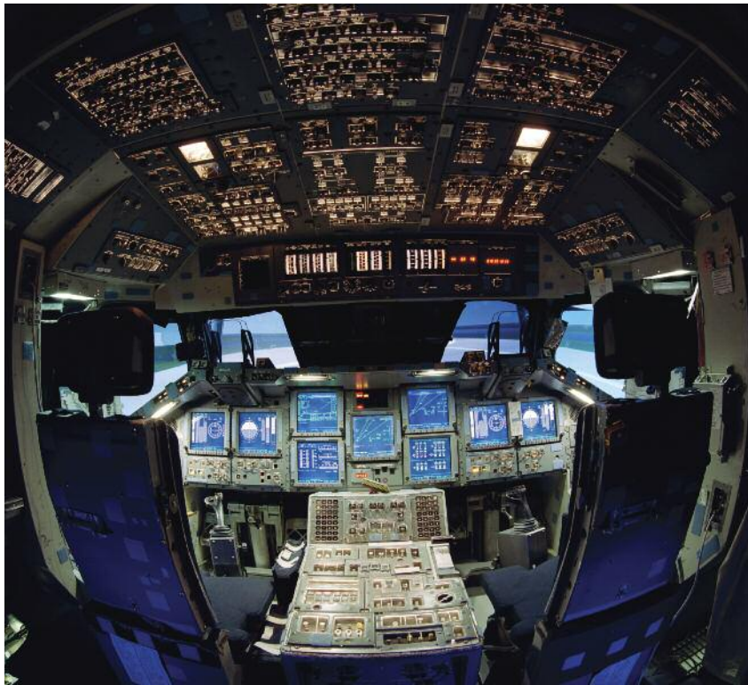
A fish-eye view of the multifunction electronic display subsystem—or “glass cockpit”—in the fixed-base Space Shuttle mission simulator at Johnson Space Center, Texas.
