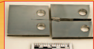
Fracture mechanics pretest and posttest specimens for characterizing material behavior.
