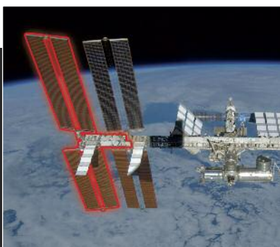
Discovery (STS-119) brought S6 truss segment.
