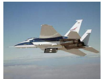
NASA validated computational fluid dynamics and flight simulation models of the foam debris in flight tests using the Dryden Flight Research Center (California) F-15B Research test bed aircraft. In these tests, debris fell from foam panels at simulated shuttle flight conditions. High-speed video cameras captured the initial flight of the foam divots.
