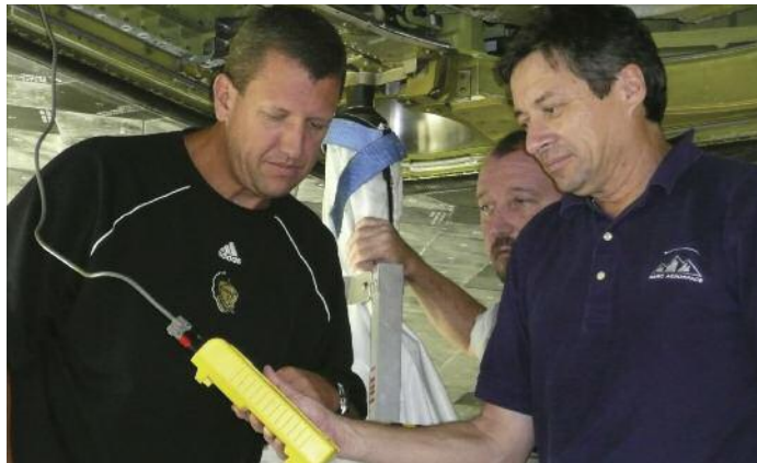
Kennedy Space Center engineers conduct wire fault testing using portable Standing Wave Reflectometer. From left to right: Ken Hosterman; John Jones; and Pedro Medelius (inventor).
