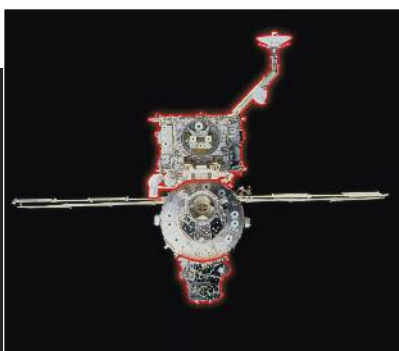
Discovery (STS-92) delivered Z1 truss and antenna (top) and one of the mating adapters.
