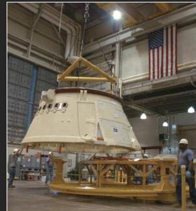
Solid Rocket Booster aft skirt processing at the Assembly and Refurbishment Facility at Kennedy Space Center.
