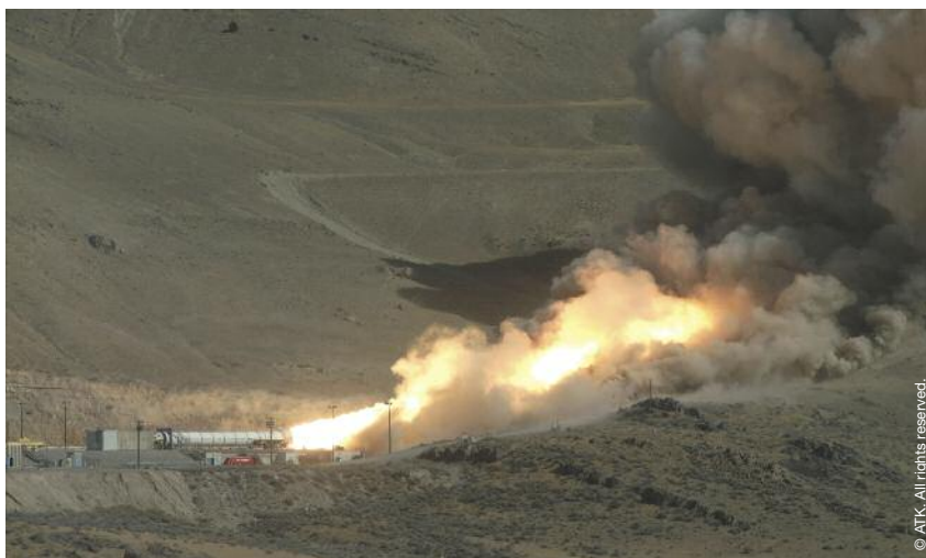
In Utah, rigorous test program included 53 reusable solid rocket motor ground tests between 1977 and 2010. Spectators flocked by the thousands to witness firsthand the equivalent of 15 million horsepower safely unleashed from a vantage point of 2 to 3 km (1 to 2 miles) away.
