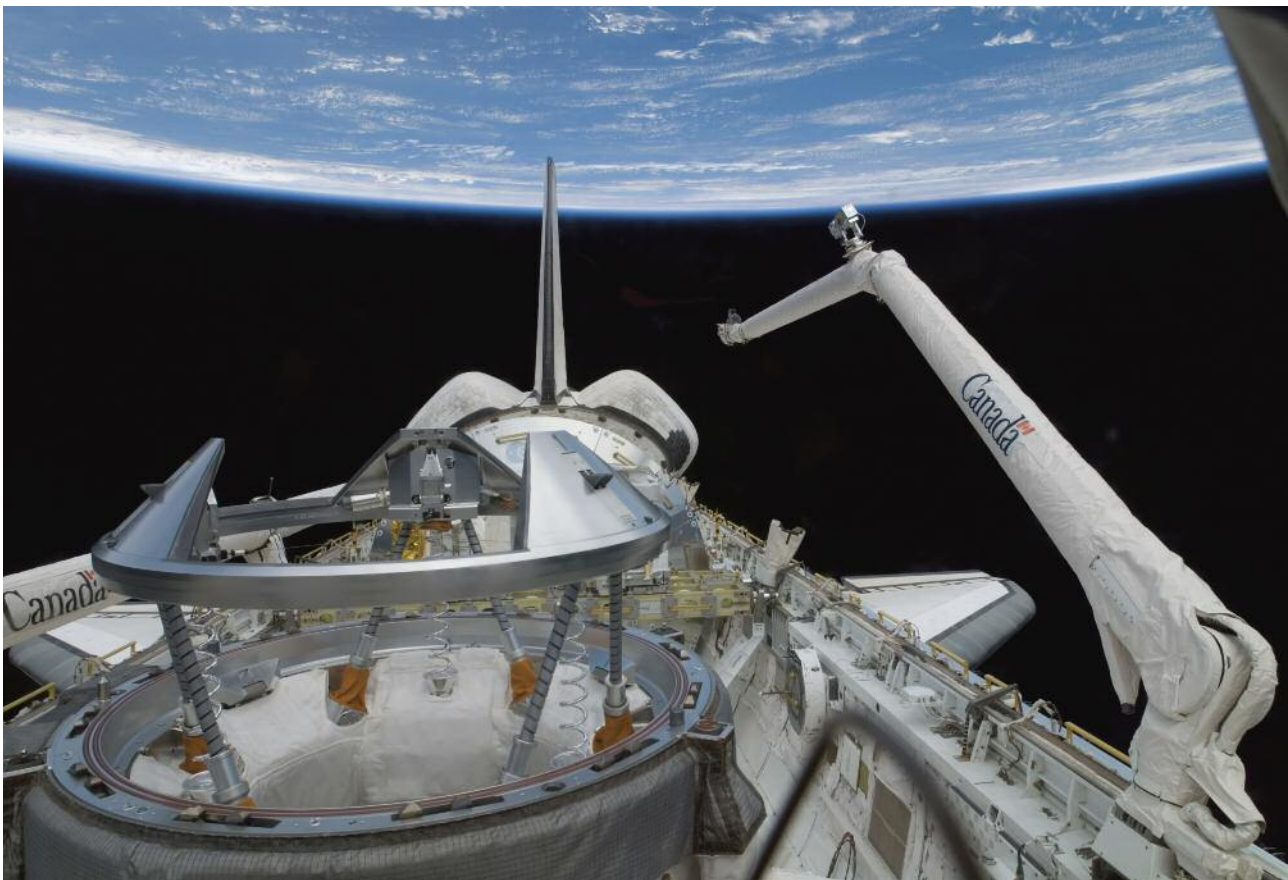
Backdropped by the blackness of space and Earth’s horizon, Atlantis’ Orbiter Docking System (foreground) and the Canadarm—the Shuttle Robotic Arm developed by Canada—in the payload bay are featured in this image photographed by an STS-122 (2008) crew member during Flight Day 2 activities.
