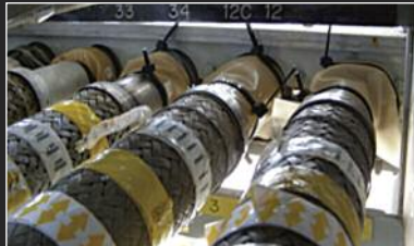
Hydrogen-sensing tape applied to the Orbiter midbody umbilical unit during fuel cell loading for STS-118 through STS-123 at Kennedy Space Center, Florida.
