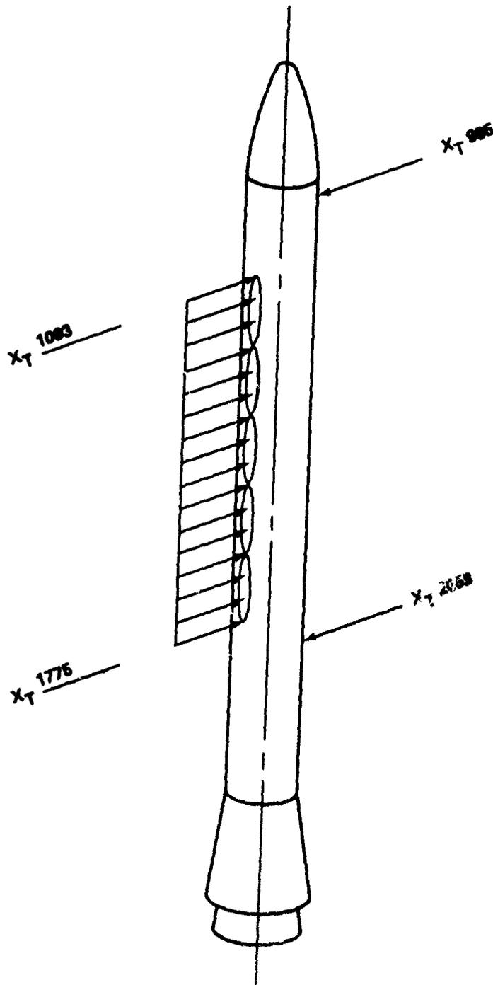
FIGURE 4-2 THRUST FROM CLAMSHELL RUPTURE
