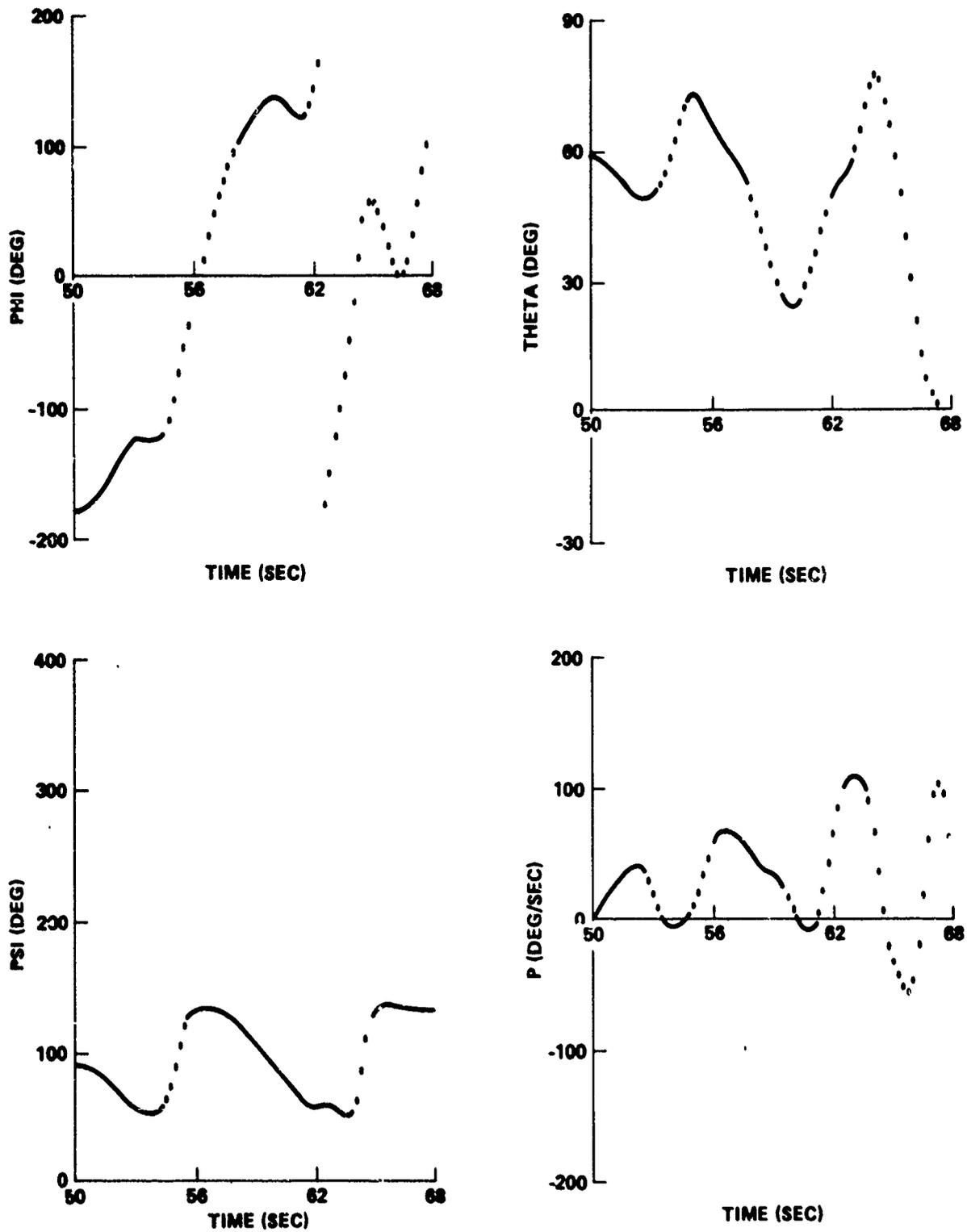
FIGURE B-14 ASCENT TRAJECTORY PARAMETERS FOR INTEGRATED VEHICLE WITH INADVERTENT RIGHT SRB SEPARATION 50 SECCNDS AFTER LIFT-OFF
