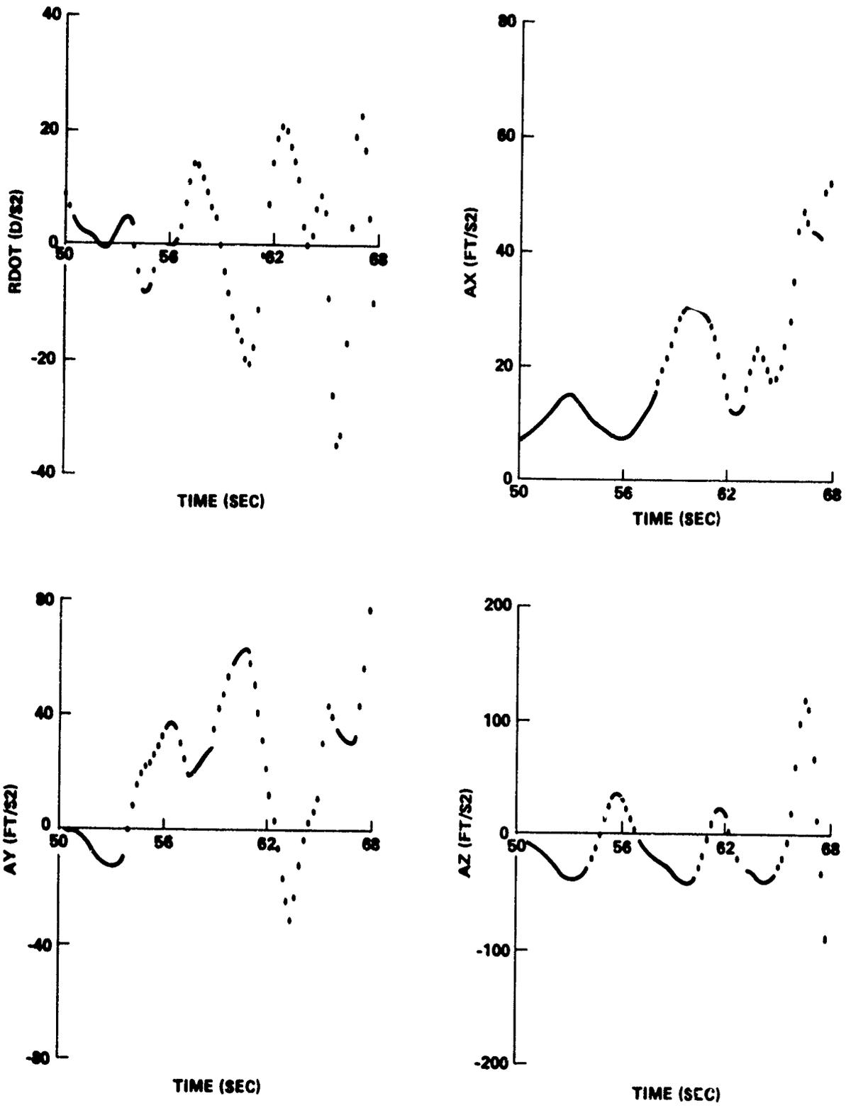
FIGURE B-16 ASCENT TRAJECTORY PARAMETEPS FOR INTEGRATED VEHICLE WITH INADVERTENT RIGHT SRB SEPARATION 50 SECONDS AFTER LIFT-OFF
