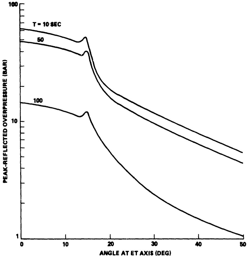
FIGURE 2-17 PEAK REFLECTED OVERPRESSURE ALONG SURFACE OF ET DUE TO EXPLOSION OF BARE SRB CHAMBER AT NORMAL OPERATING PRESSURE
