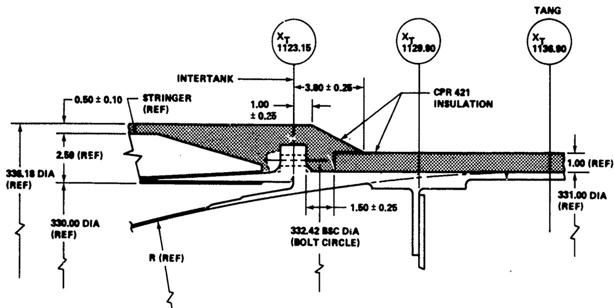
FIGURE K-3 OUTER CHORD -- FRAME X<sub>T</sub> 1129.9
