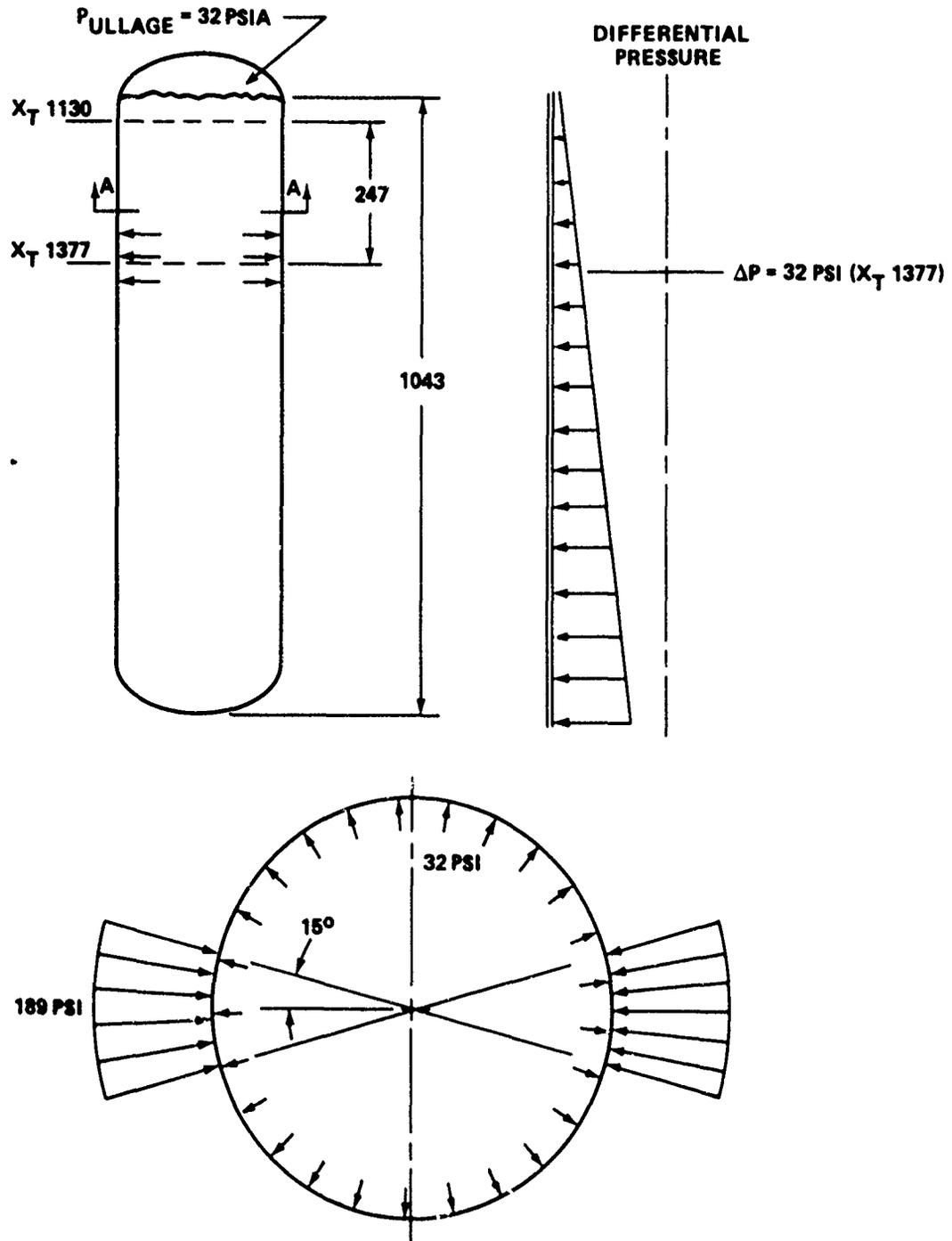
FIGURE 4-44 EXTERNAL BLAST PRESSURE AND INTERNAL PRESSURE AT T = 100 SECONDS
