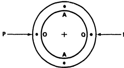
If we assume rigid plastic stress-strain behavior, an estimate of the collapse load can be made. Let us first compute the load  $P_y$  to yield the structure. By symmetry, we need only analyze 1/4 of the frame.
