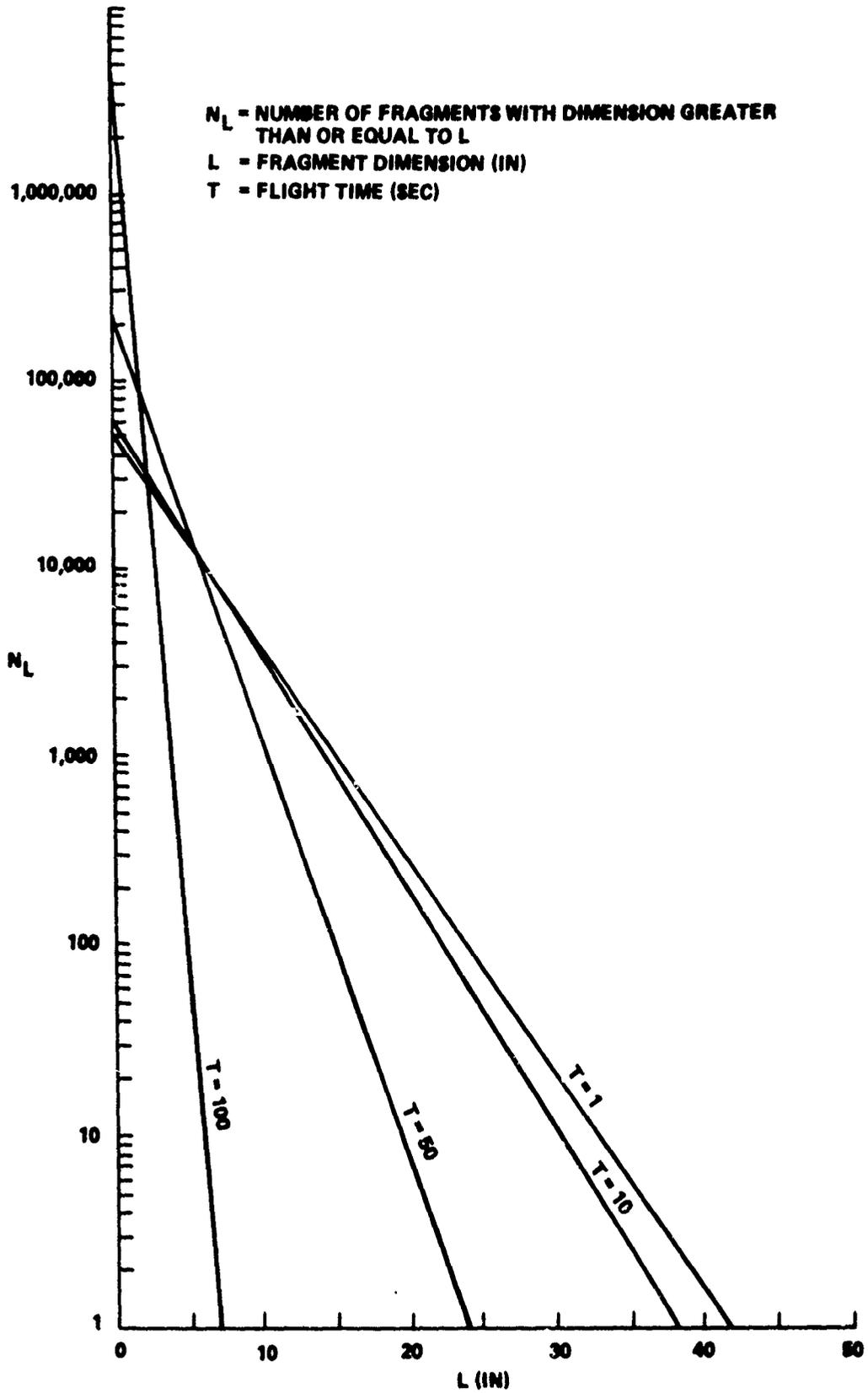
FIGURE 2-11 FRAGMENT SIZE DISTRIBUTION FUNCTION FOR PROPELLANT
