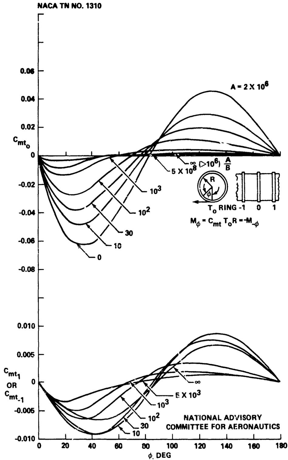
FIGURE 4-67 RING BENDING-MOMENT COEFFICIENTS FOR TANGENTIAL LOAD
