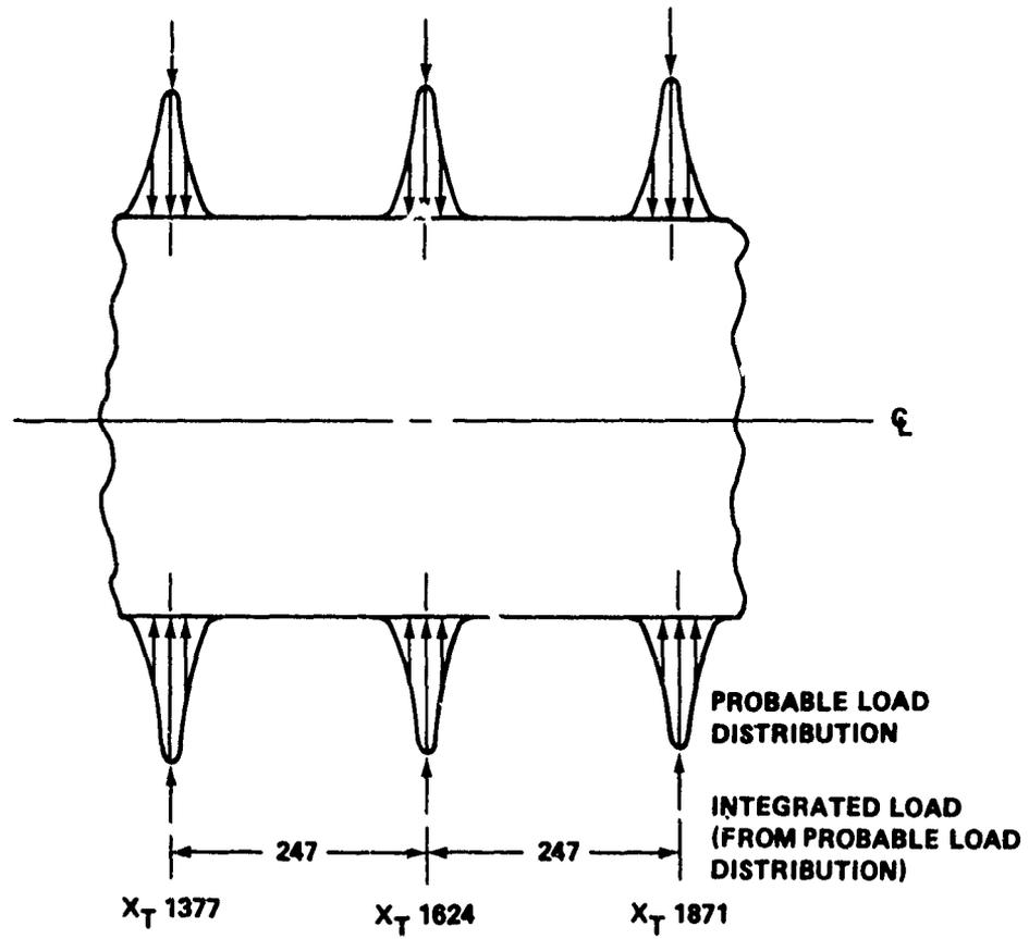
FIGURE I-2 STRUCTURAL MODEL FOR ET TANK (PLAN VIEW)
