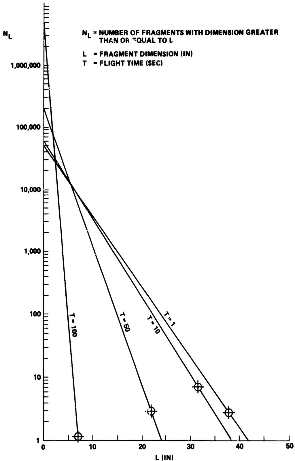
FIGURE 4-39 FRAGMENT SIZE DISTRIBUTION FUNCTION FOR PROPELLANT
