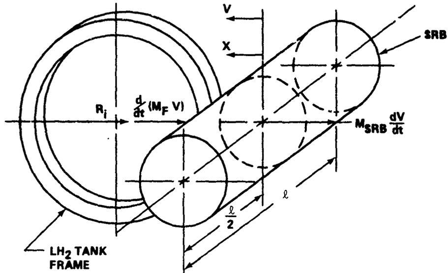
FIGURE 4-27 SECTION OF SRB IMPACTING A SECTION OF LH<sub>2</sub> TANK SUPPORTED BY AN INTERNAL RING FRAME
