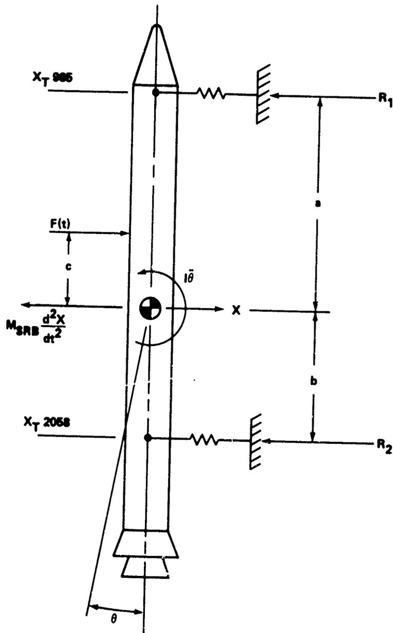
FIGURE 4-24 FORCES ACTING ON SRB DURING DESTRUCT
