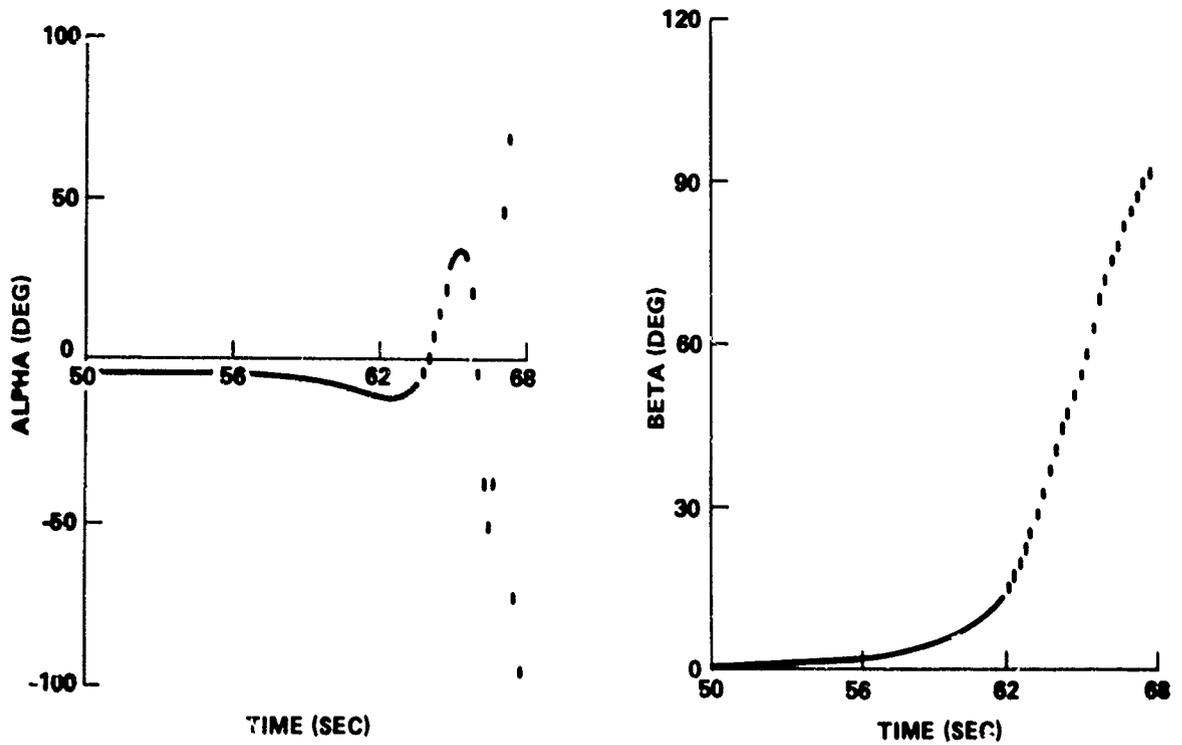
FIGURE B-37 ASCENT TRAJECTORY PARAMETERS FOR INTEGRATED VEHICLE WITH INADVERTENT ORBITER SEPARATION 50 SECONDS AFTER LIFT-OFF
