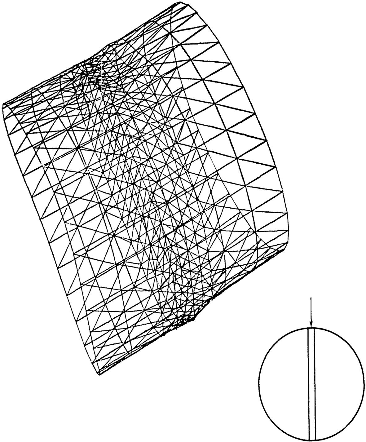
FIGURE 4-51 FINITE ELEMENT MODEL OF ET INTERTANK STRUCTURE
