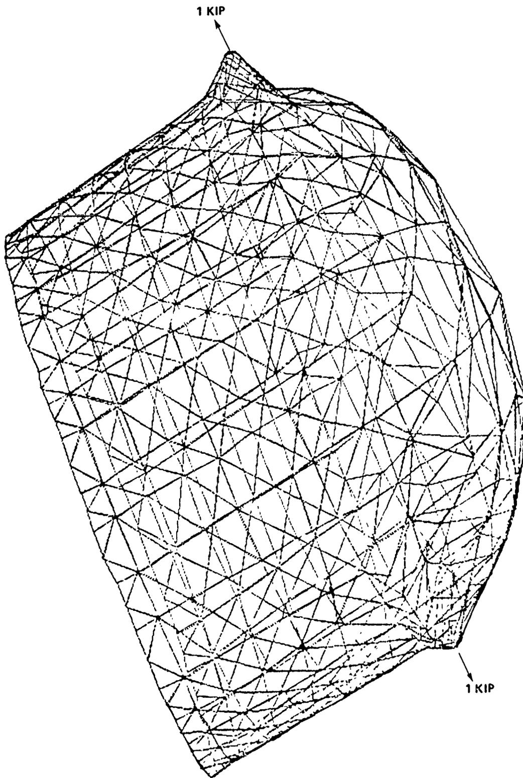
FIGURE C-7 STATIC ANALYSIS OF ET RING FRAME LOCATED AT STATION X<sub>T</sub> 2058
