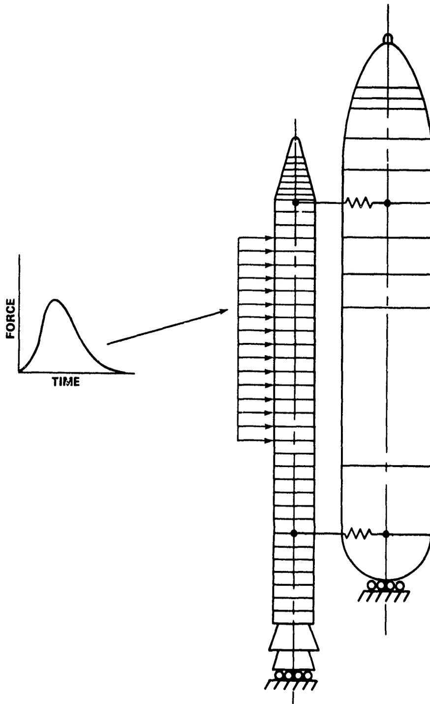
FIGURE 4-48 FINITE ELEMENT MODEL FOR RESPONSE DUE TO LATERAL THRUST OF ONE SRB
