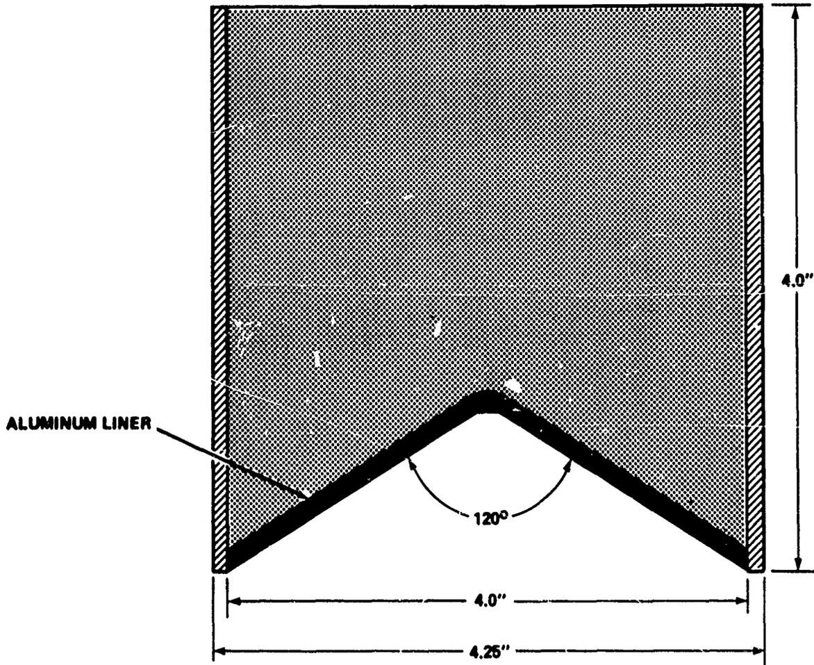
FIGURE 2-20 120-DEGREE CONICAL LINER
