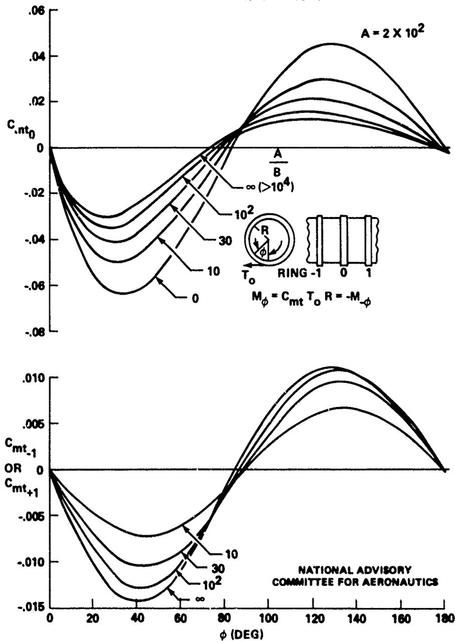
FIGURE K-9 RING BENDING-MOMENT COEFFICIENTS FOR TANGENTIAL LOAD
