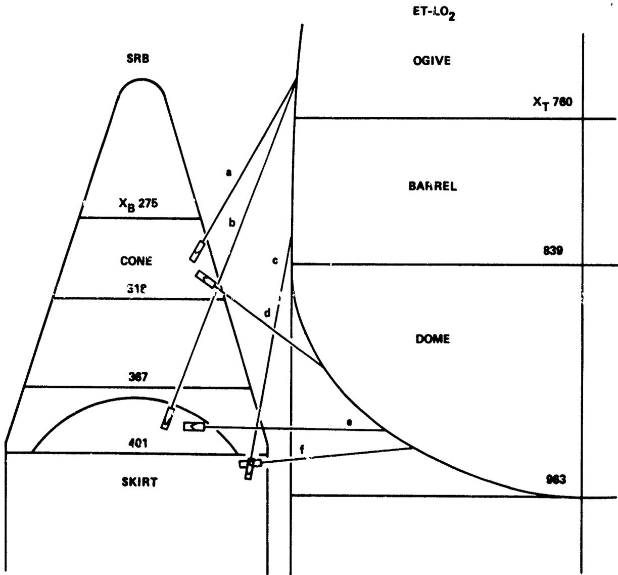
FIGURE 2-21 ET-LO<sub>2</sub> DESTRUCT TRAJECTORY OPTIONS FOR SHAPED CHARGE JETS
