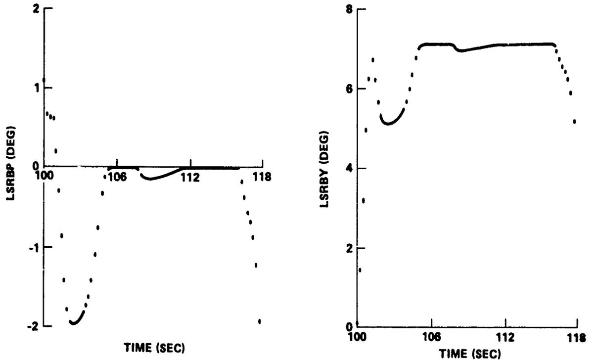
FIGURE B-25 ASCENT TRAJECTORY PARAMETERS FOR INTEGRATED VEHICLE WITH INADVERTENT RIGHT SRB SEPARATION 100 SECONDS AFTER LIFT-OFF
