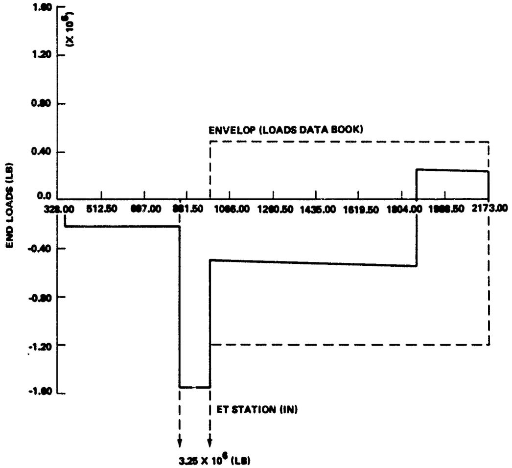
FIGURE J-5 ET END LOAD (T = 51.75 SEC) FOLLOWING LOSS OF SRB AT 50 SECONDS
