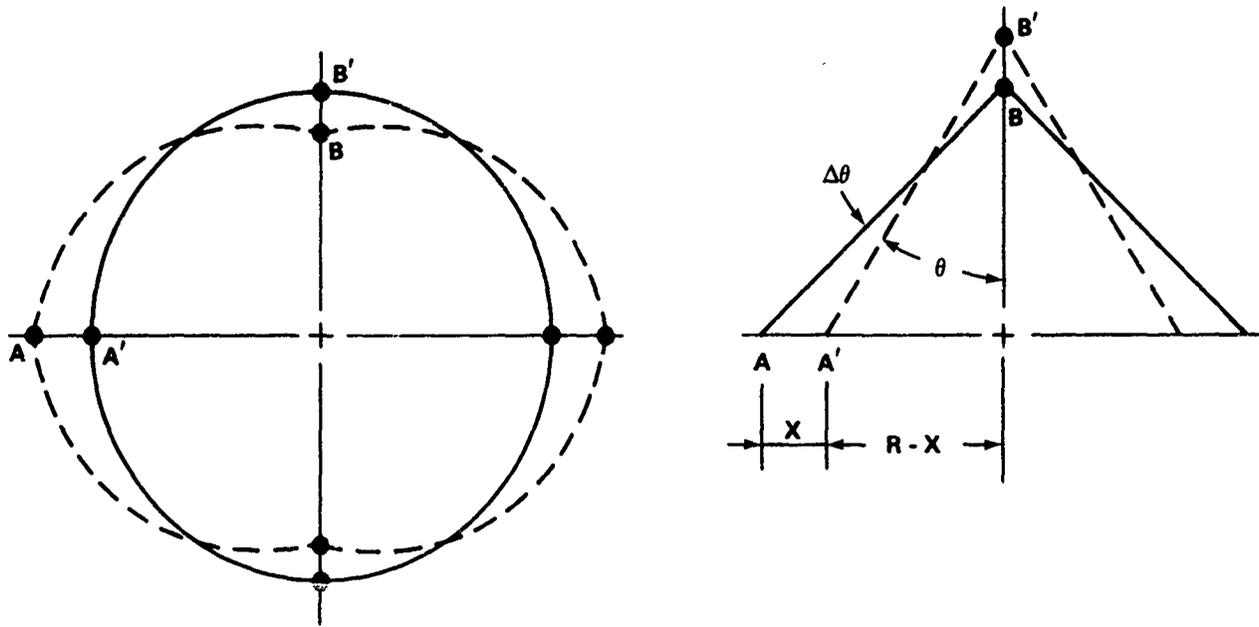
Assume the hinges rotate through an angle of  $\Delta\theta$  as the frame deflects from A to A'. Further assume that the frame length  $AB = A'B' = \sqrt{2} R$ . Then
