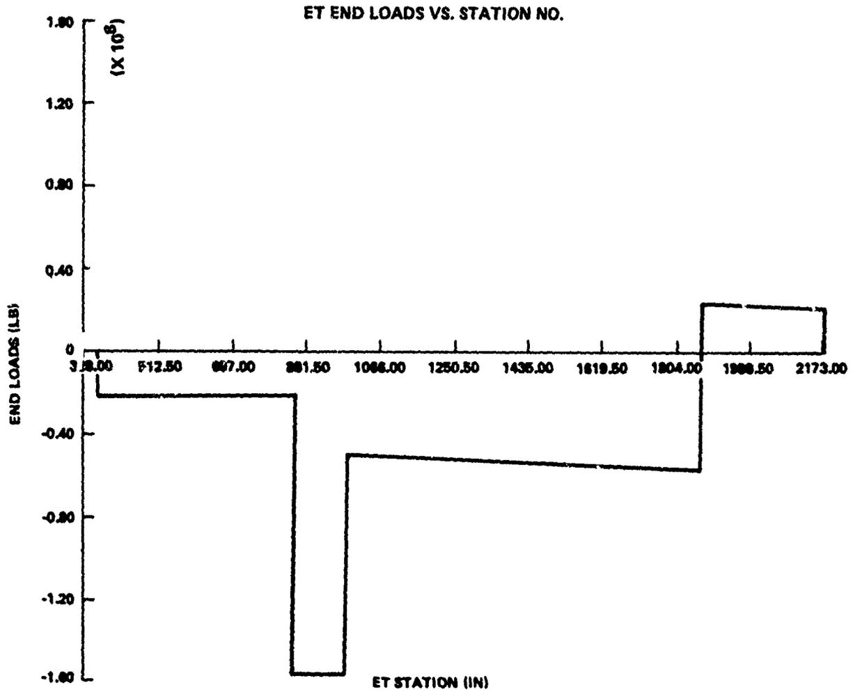
FIGURE 4-83 ET END LOAD (T = 51.75 SEC) FOLLOWING LOSS OF SRB AT 50 SECONDS
