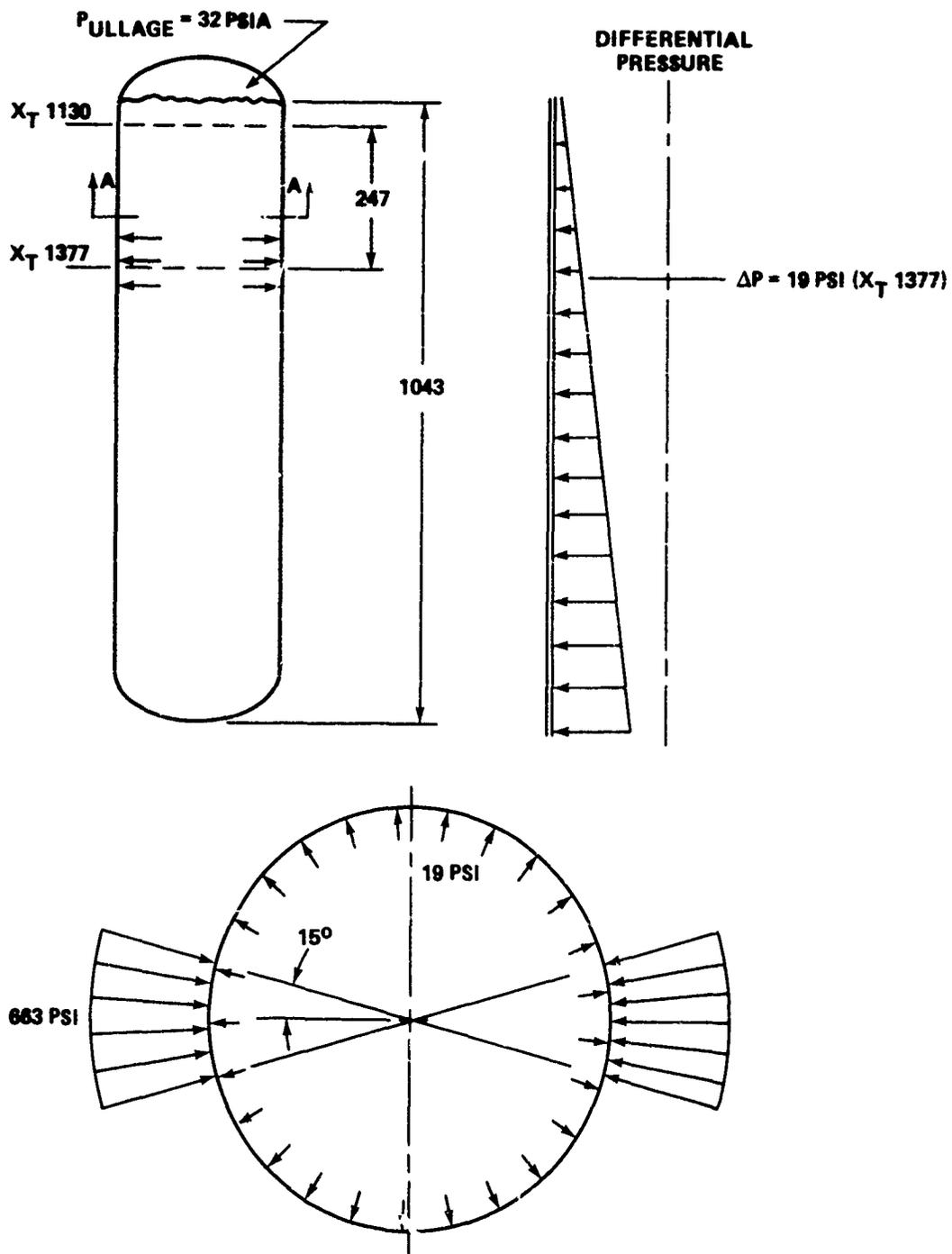
FIGURE 4-43 EXTERNAL BLAST PRESSURE AND INTERNAL PRESSURE AT  $T = 10$  SECONDS
