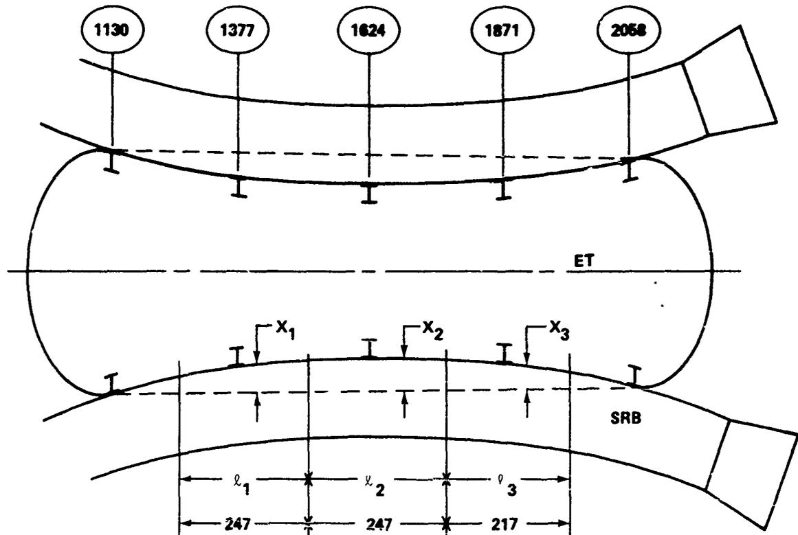
FIGURE 4-33 DEFORMED SHAPE OF LH<sub>2</sub> TANK
