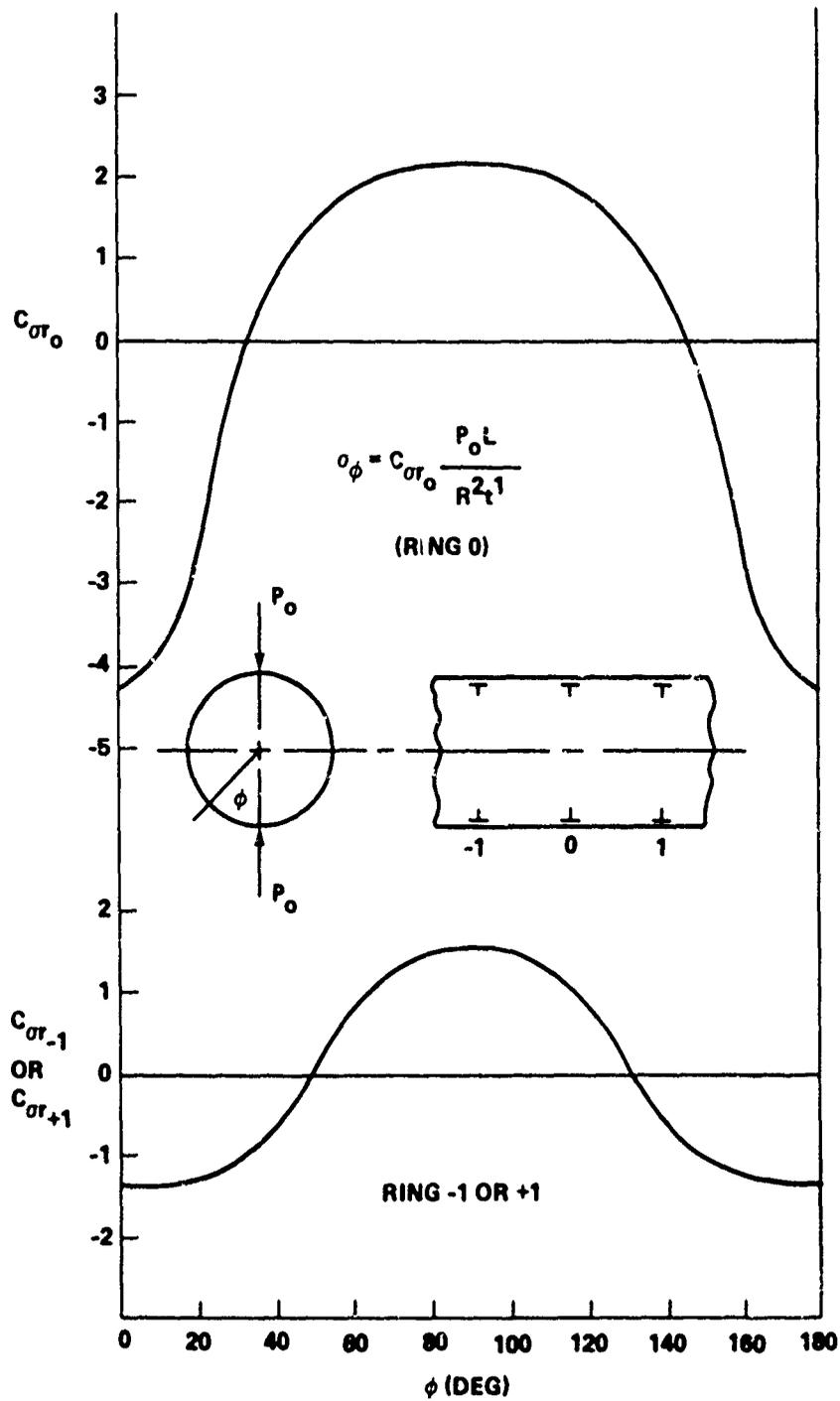
FIGURE I-5 SKIN-DIRECT STRESS COEFFICIENTS AT RINGS FOR RADIAL LOADS
