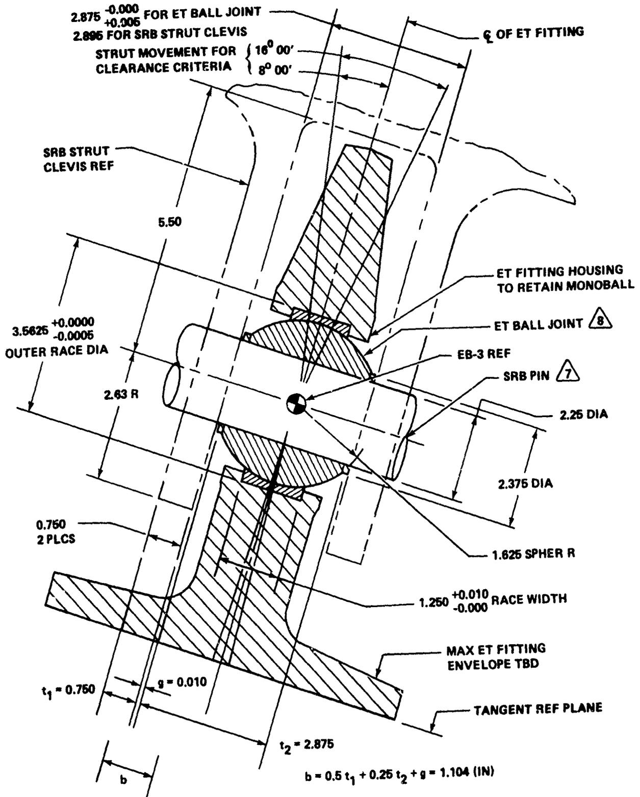
FIGURE 4-71 CLEVIS JOINT - SRB/ET AFT STRUT
