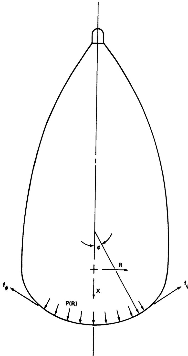
FIGURE 4-58 LOADING ON LOX TANK DOME
