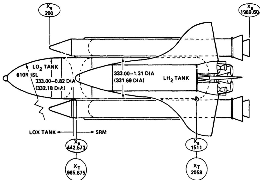
FIGURE 4-56 RELATIVE LOCATION OF LOX TANK TO SRM
