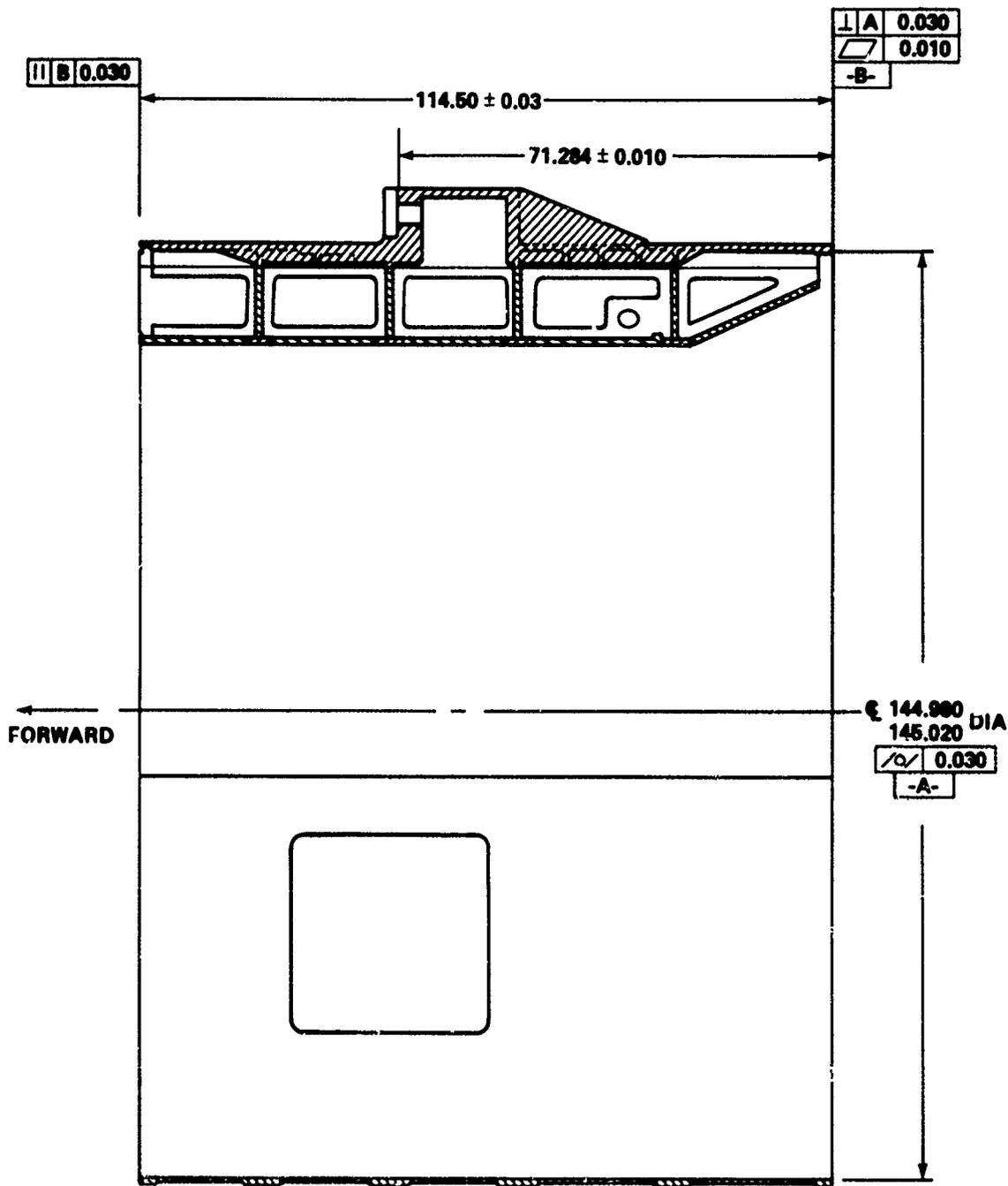
FIGURE F-3 THRUST POST FITTING AND BOX BEAM
