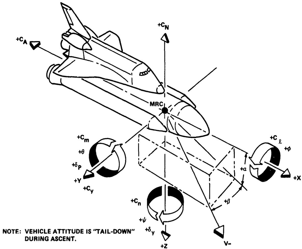
FIGURE B-1 ASCENT VEHICLE AXIS SYSTEM
