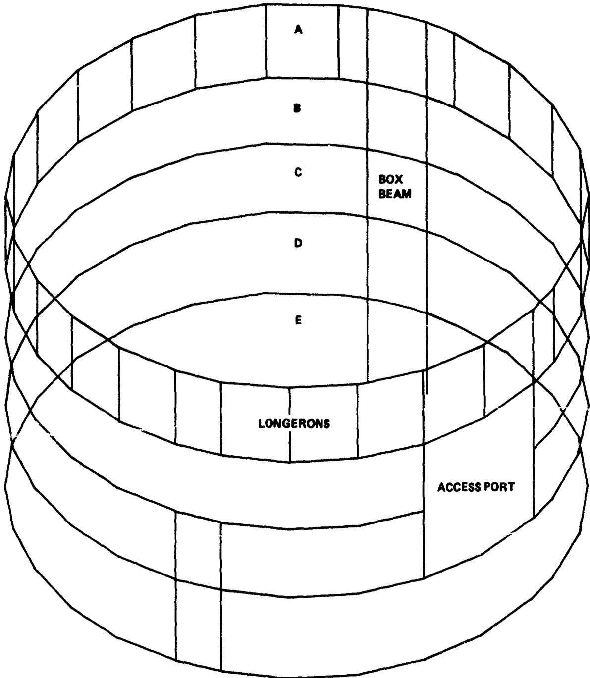
FIGURE F-6 FINITE ELEMENT MODEL OF RING FRAMES, BOX BEAM, AND LONGERONS
