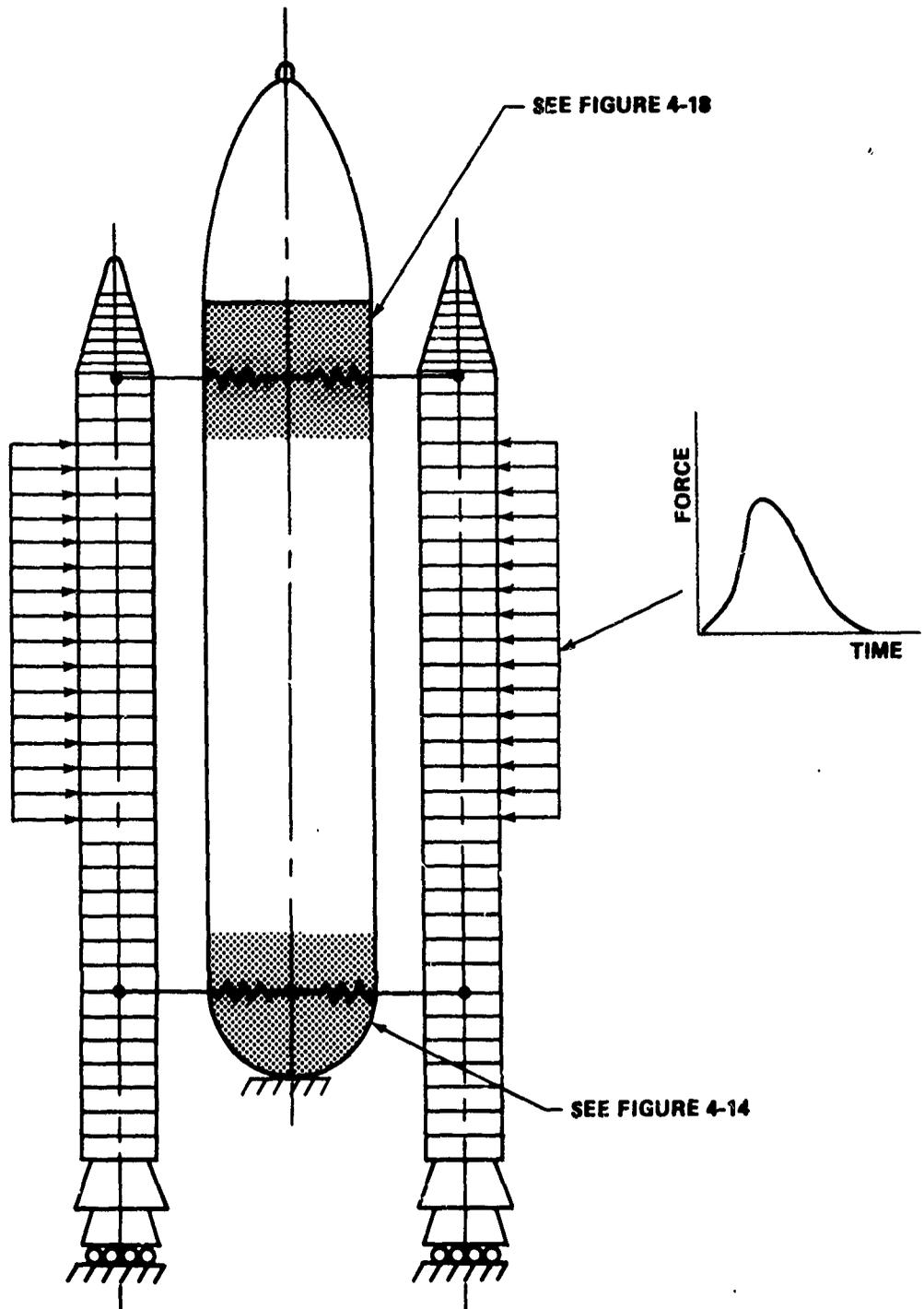
FIGURE 4-4 FINITE ELEMENT MODEL FOR RESPONSE DUE TO LATERAL THRUST
