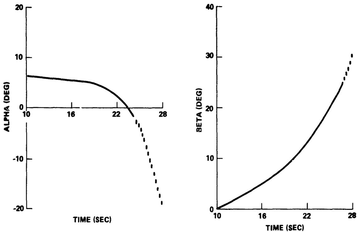
FIGURE B-33 ASCENT TRAJECTORY PARAMETERS FOR INTEGRATED VEHICLE WITH INADVERTENT ORBITER SEPARATION 10 SECONDS AFTER LIFT-OFF
