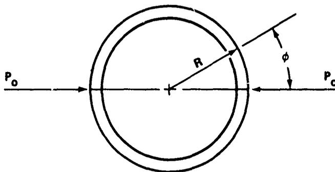
FIGURE 4-29 RESISTANCE FOR RING LOADED BY TWO RADIAL LOADS
