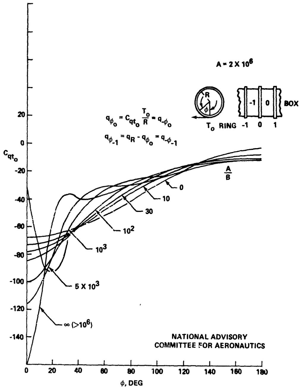
FIGURE 4-68 SKIN SHEAR-FLOW COEFFICIENTS FOR TANGENTIAL LOAD
