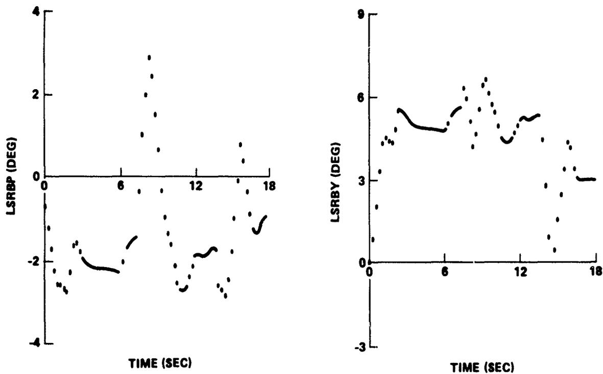
FIGURE B-7 ASCENT TRAJECTORY PARAMETERS FOR INTEGRATED VEHICLE WITH INADVERTENT RIGHT SRB SEPARATION AT LIFT-OFF
