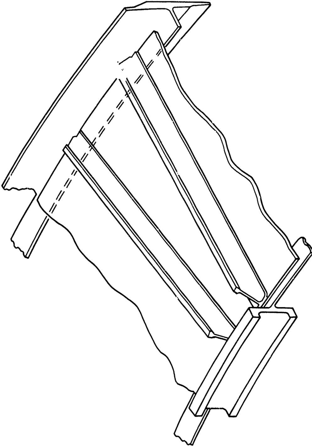
FIGURE C-1 ET RING FRAME AT STATION  $X_T$  2058
