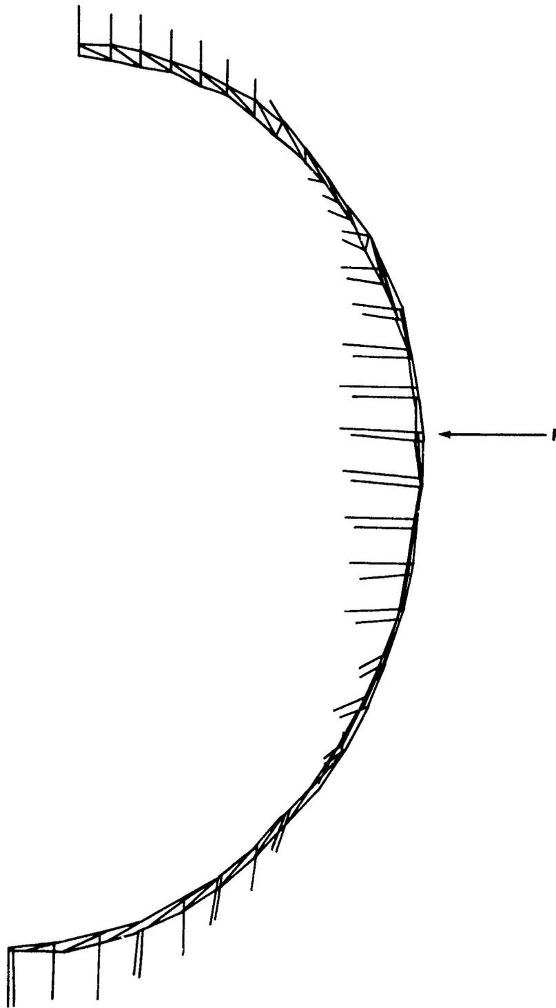
FIGURE E-11 DEFORMED SHAPE — FRAME  $X_T$  985
