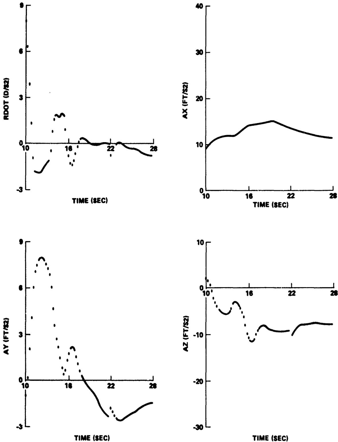
FIGURE B-10 ASCENT TRAJECTORY PARAMETERS FOR INTEGRATED VEHICLE WITH INADVERTENT RIGHT SRB SEPARATION 10 SECONDS AFTER LIFT-OFF
