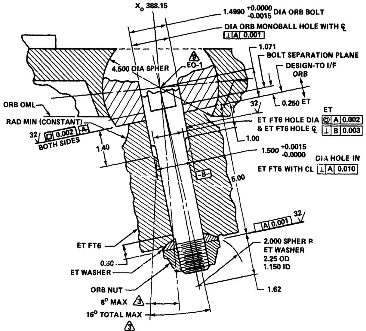
FIGURE 4-79 ORBITER SEPARATION BOLT
