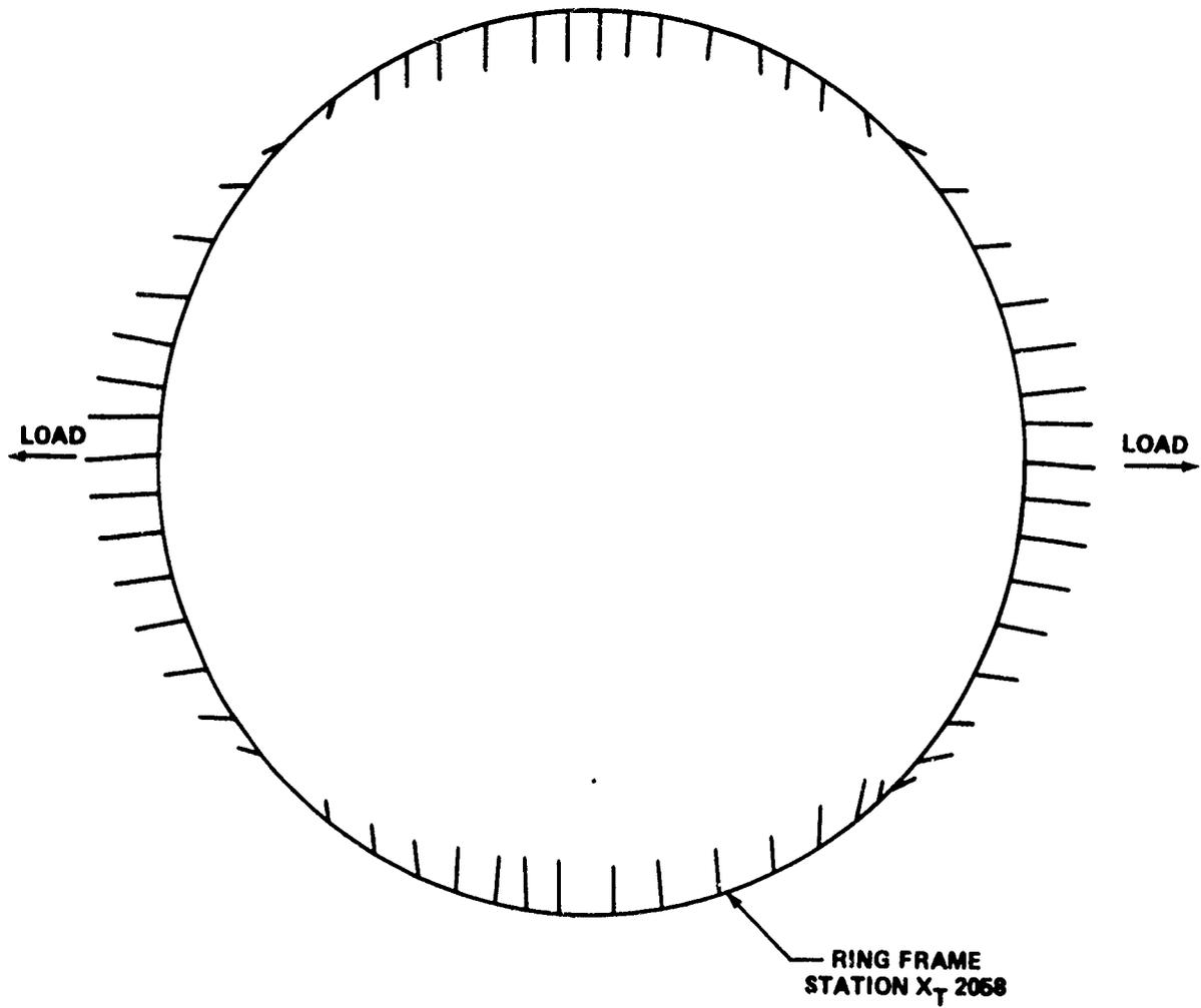
FIGURE C-8 DEFLECTION PATTERN - TEST CASE
