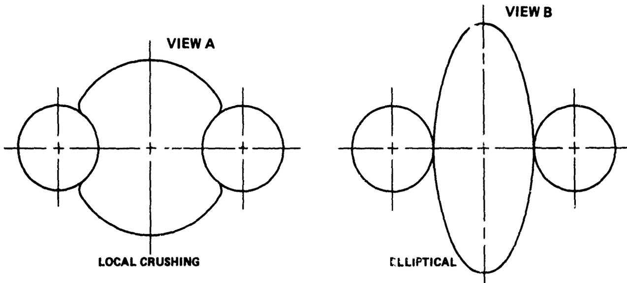
FIGURE 4-28 DEFORMED SHAPE OF LH<sub>2</sub> TANK FRAMES BOUNDED BY TWO EXTREMES
