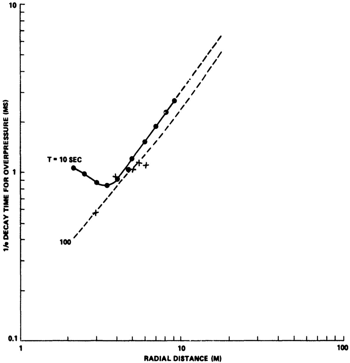
FIGURE 2-15 1/e DECAY TIME FOR FREE-AIR OVERPRESSURE VS. RADIAL DISTANCE FROM SRB AXIS
