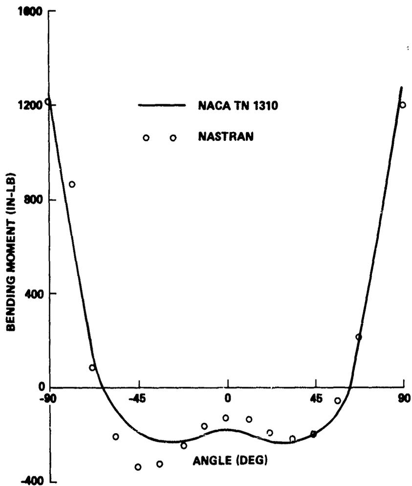
FIGURE E-8 TEST CASE - BENDING MOMENT IN FRAME X<sub>T</sub> 985.7
