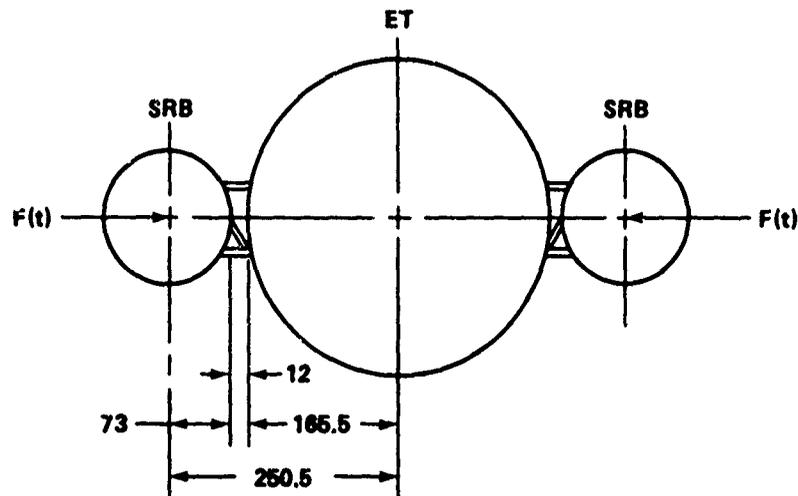
FIGURE 4-1 ET/SRB GEOMETRY
