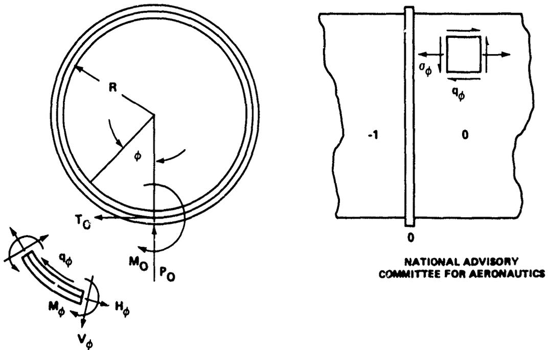
FIGURE I-3 STRUCTURAL MODEL FOR ET UNDER RADIAL LOADS
