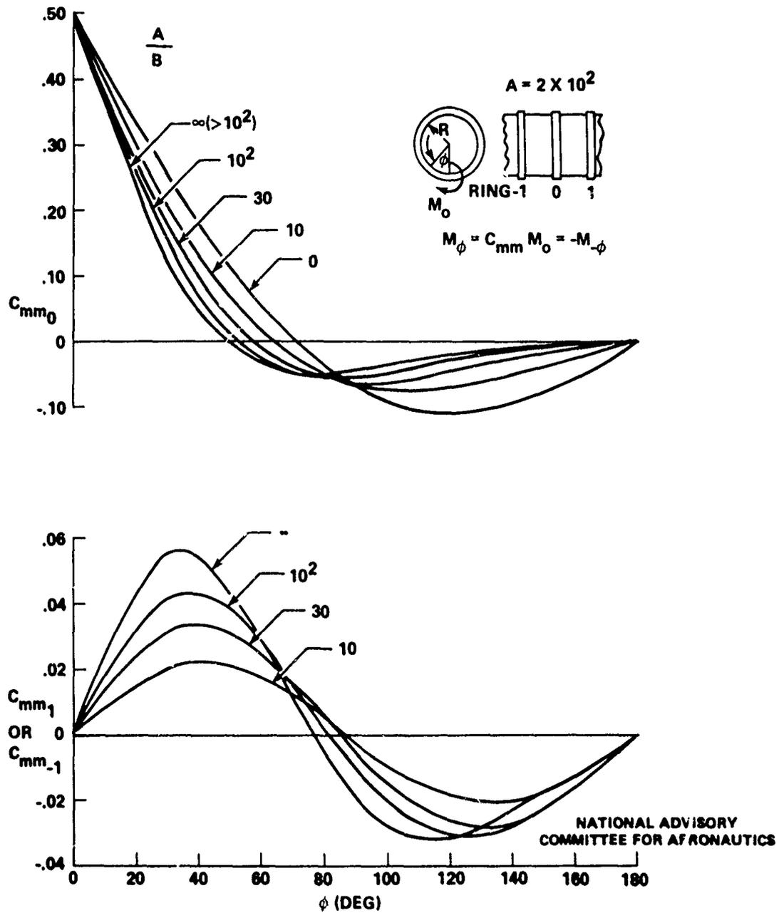
FIGURE K-10 RING BENDING-MOMENT COEFFICIENTS FOR MOMENT LOAD
