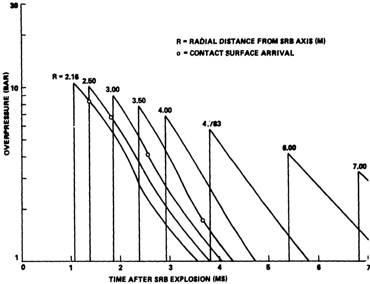
FIGURE 2-14 FREE-AIR PRESSURE VS. TIME AT VARIOUS DISTANCES FROM AXIS OF BARE 827 PSIA SRB CHAMBER EXPLODED AT T = 10 SECONDS
