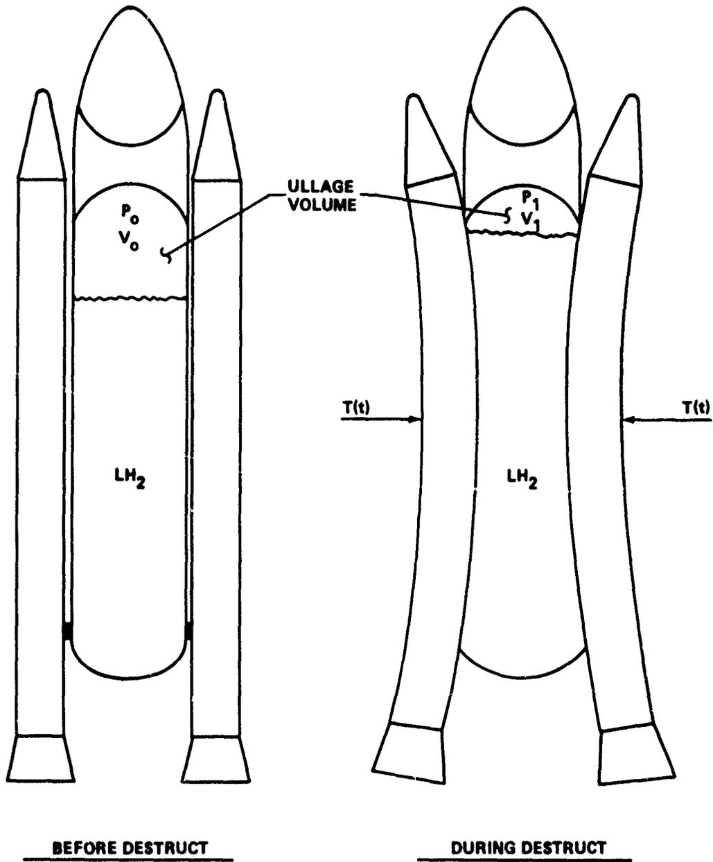
FIGURE 4-26 COMPRESSION OF ULLAGE VOLUME DURING DESTRUCT
