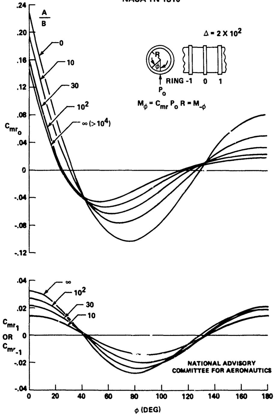
FIGURE K-8 RING BENDING-MOMENT COEFFICIENTS FOR RADIAL LOAD
