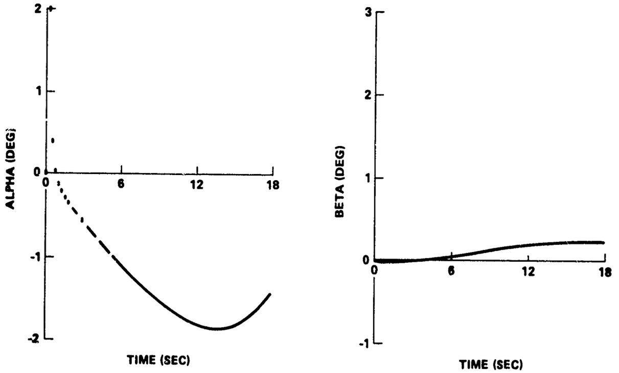
FIGURE B-29 ASCENT TRAJECTORY PARAMETERS FOR INTEGRATED VEHICLE WITH INADVERTENT ORBITER SEPARATION AT LIFT-OFF
