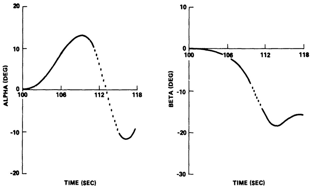
FIGURE B-41 ASCENT TRAJECTORY PARAMETERS FOR INTEGRATED VEHICLE WITH INADVERTENT ORBITER SEPARATION 100 SECONDS AFTER LIFT-OFF
