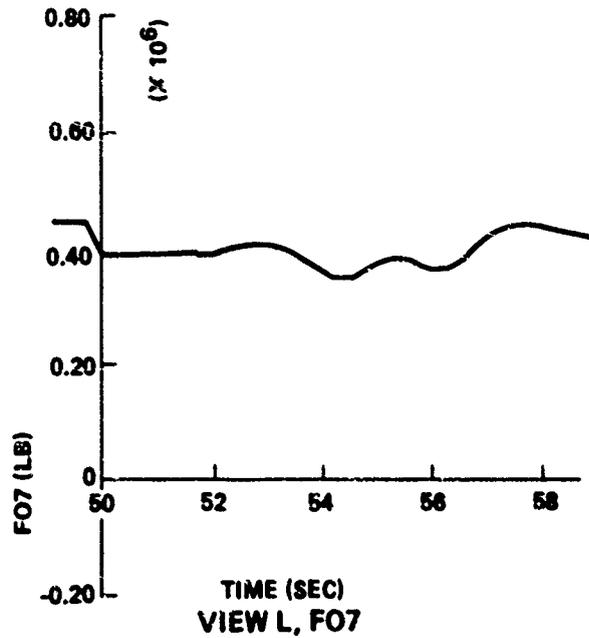
FIGURE 4-80 ATTACH FITTING LOADS - LOSS OF SRB AT 50 SECONDS (Sheet 3 of 3)
