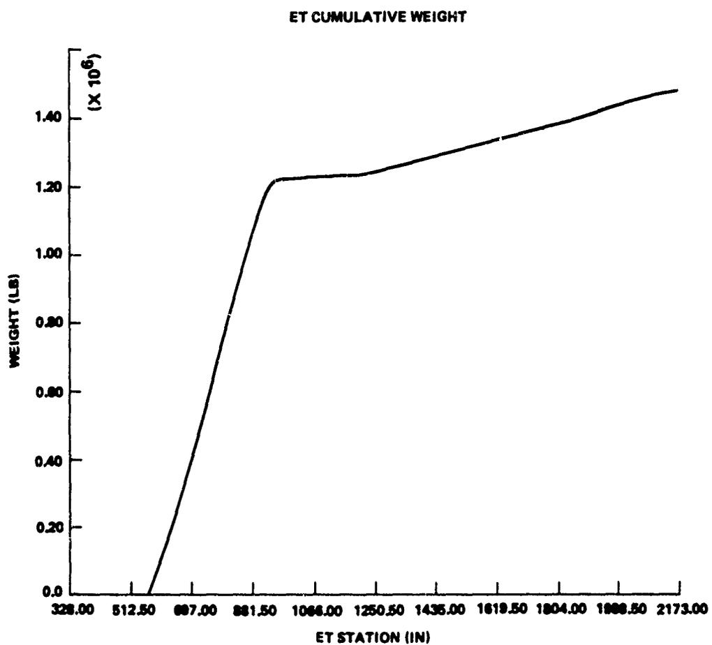
FIGURE J-4 ET CUMULATIVE WEIGHT (T = 51.75 SEC)
