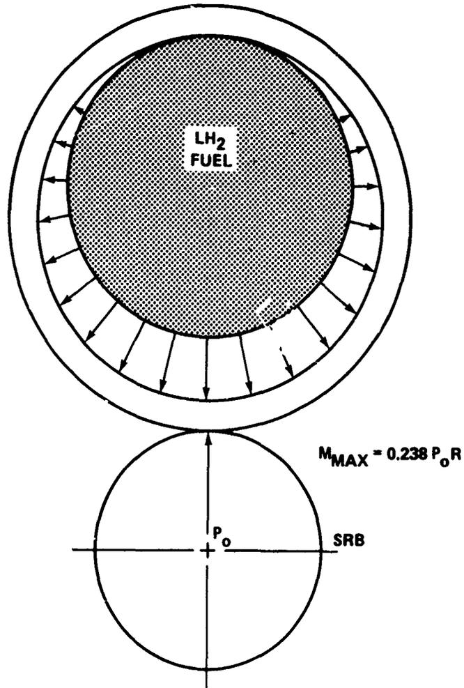
FIGURE 4-52 LOADING ON ET FRAMES DURING DESTRUCT (LOSS OF 1 SRB)
