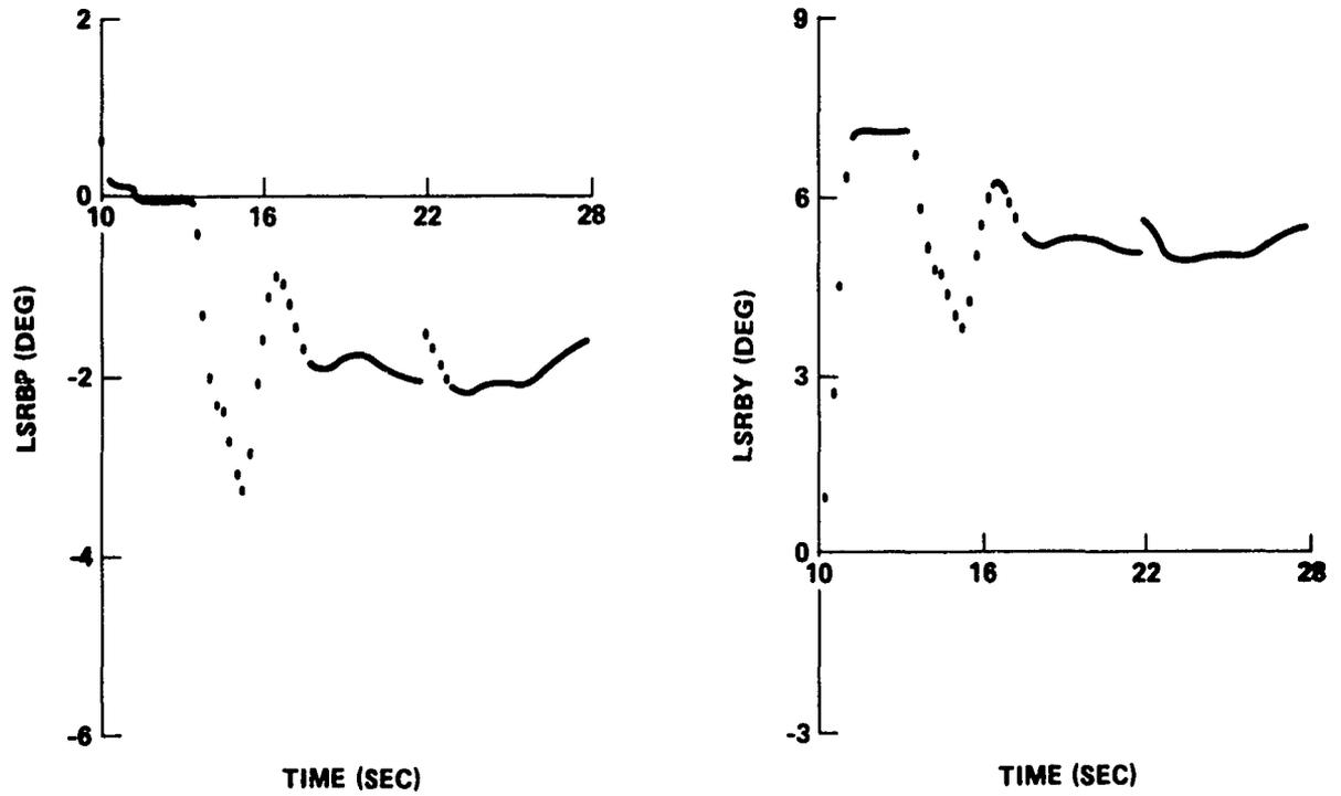
FIGURE B-13 ASCENT TRAJECTORY PARAMETERS FOR INTEGRATED VEHICLE WITH INADVERTENT RIGHT SRB SEPARATION 10 SECONDS AFTER LIFT-OFF
