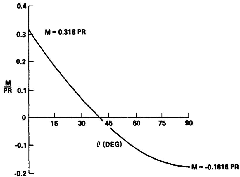
The maximum moment occurs at  $\theta = 0$ . This is where the plastic hinge forms. By limit analysis let  $M_p$  be the moment to make the cross section go completely plastic. Hence, the force to initiate a plastic hinge at point 0 is:
