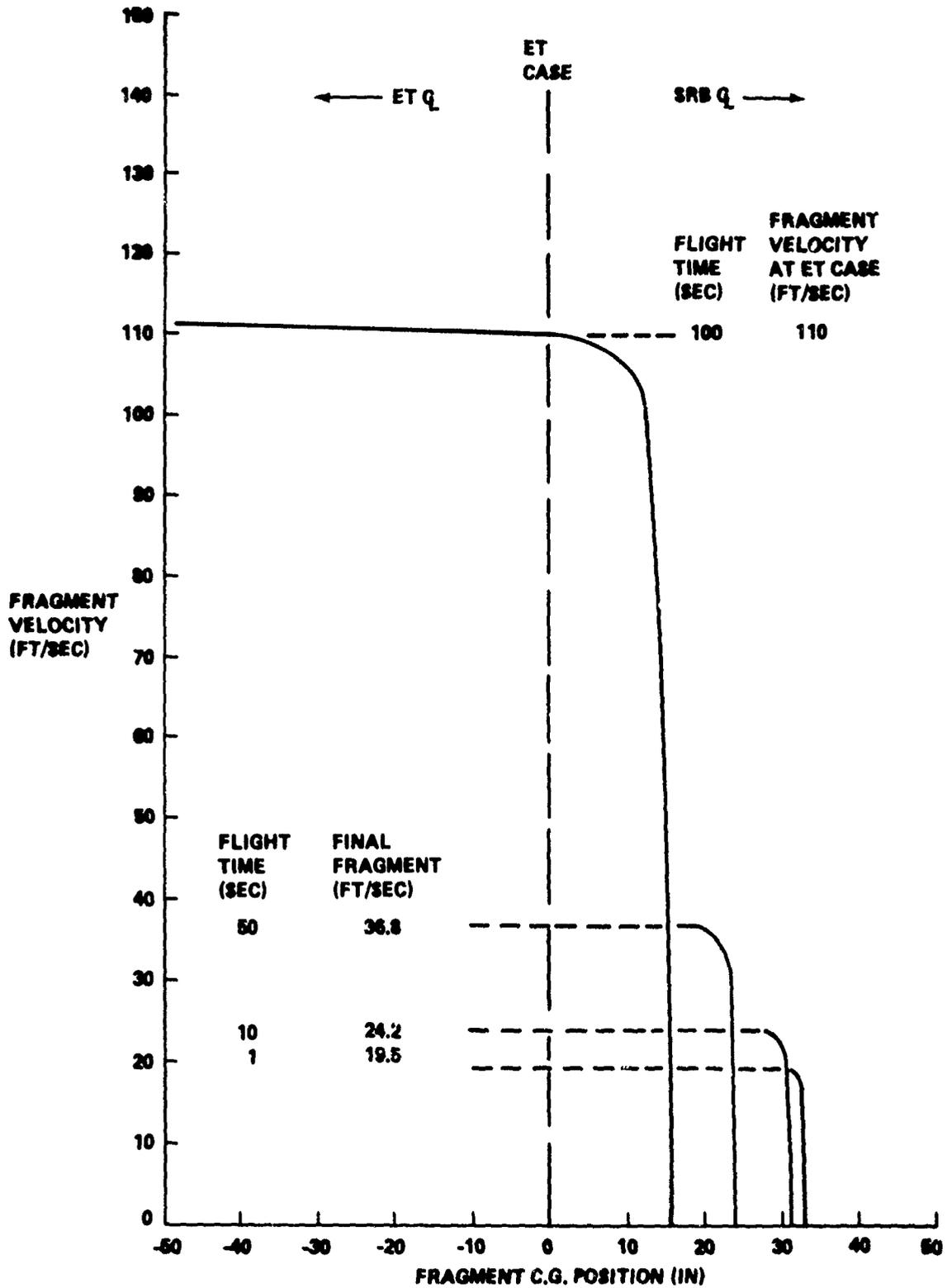
FIGURE 2-12 PROPELLANT FRAGMENT VELOCITY VS. POSITION
