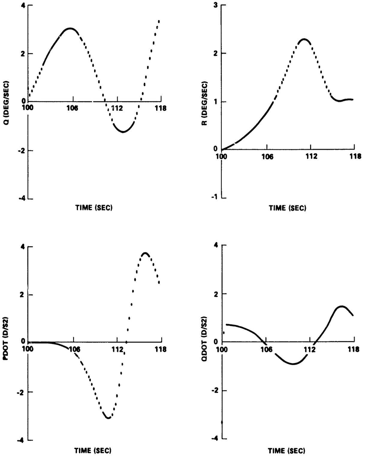
FIGURE B-39 ASCENT TRAJECTORY PARAMETERS FOR INTEGRATED VEHICLE WITH INADVERTENT ORBITER SEPARATION 100 SECONDS AFTER LIFT-OFF
