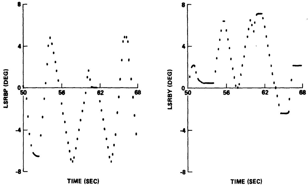
FIGURE B-19 ASCENT TRAJECTORY PARAMETERS FOR INTEGRATED VEHICLE WITH INADVERTENT RIGHT SRB SEPARATION 50 SECONDS AFTER LIFT-OFF
