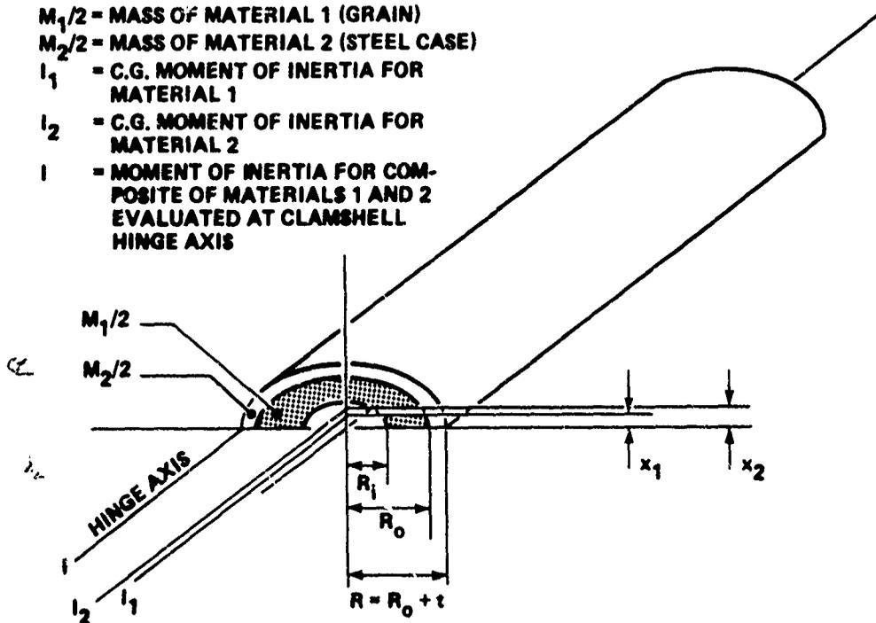
FIGURE 2-4 HALF CLAMSHELL GEOMETRY
