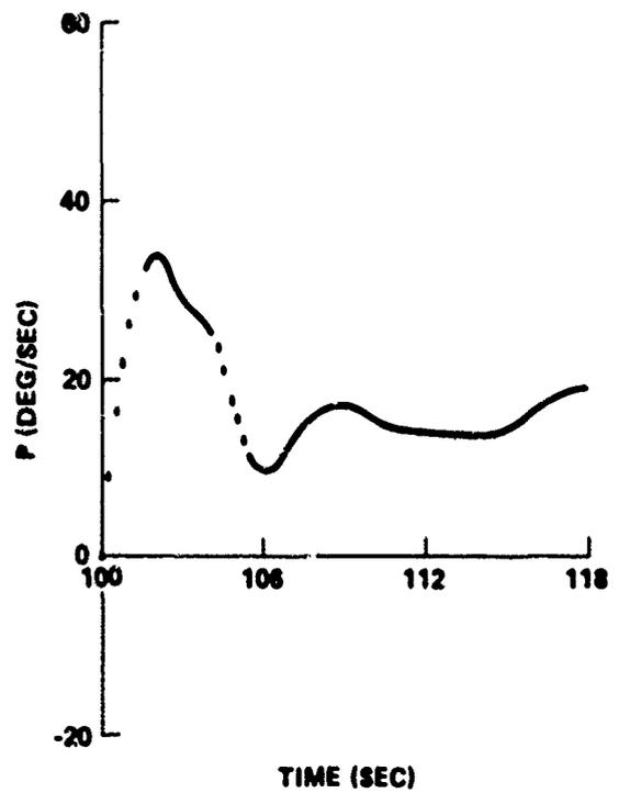
FIGURE B-20 ASCENT TRAJECTORY PARAMETERS FOR INTEGRATED VEHICLE WITH INADVERTENT RIGHT SRB SEPARATION 100 SECONDS AFTER LIFT-OFF
