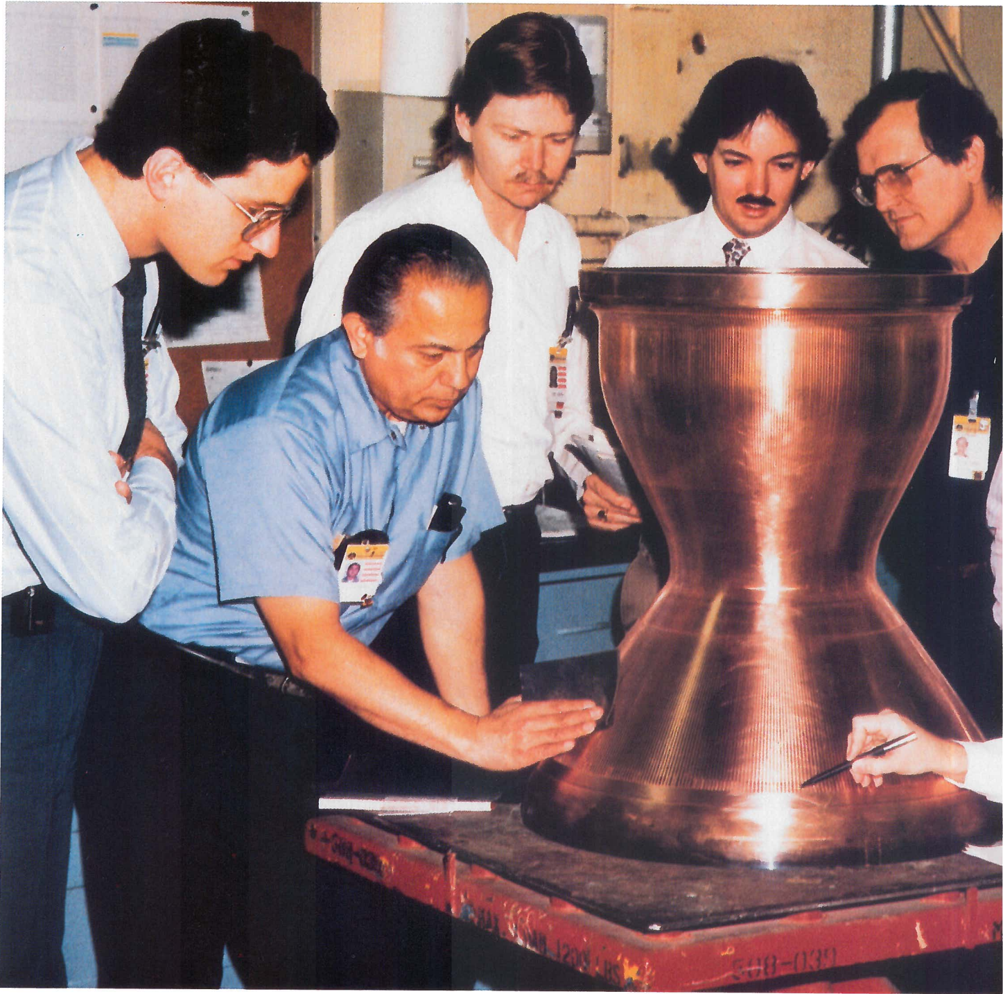
Members of one of Rocketdyne's original TQM groups, the CPI—continuous process improvement—team for SSME main combustion chamber plating, examine their work.
