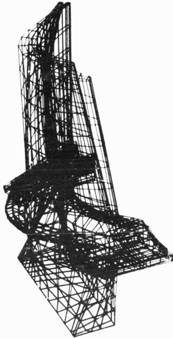
Fig. 2-7 Model F-1, Mode 3, Freq 12186
