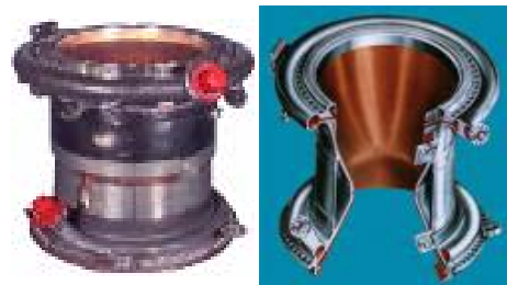
Figure 8. Large Throat Main Combustion Chamber
