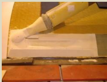
Remove/Replace Longeron Closeouts
