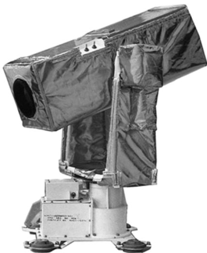
Pan/Tilt Unit and Camera with Thermal Blankets
