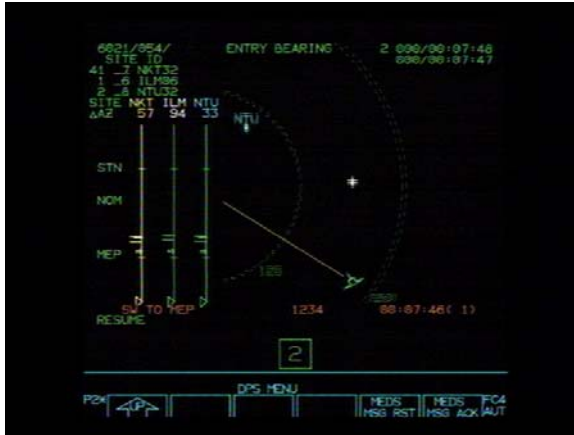
ECAL Entry to Cherry Point (NKT) with High \Delta Az - MM602 Post Nz Hold
