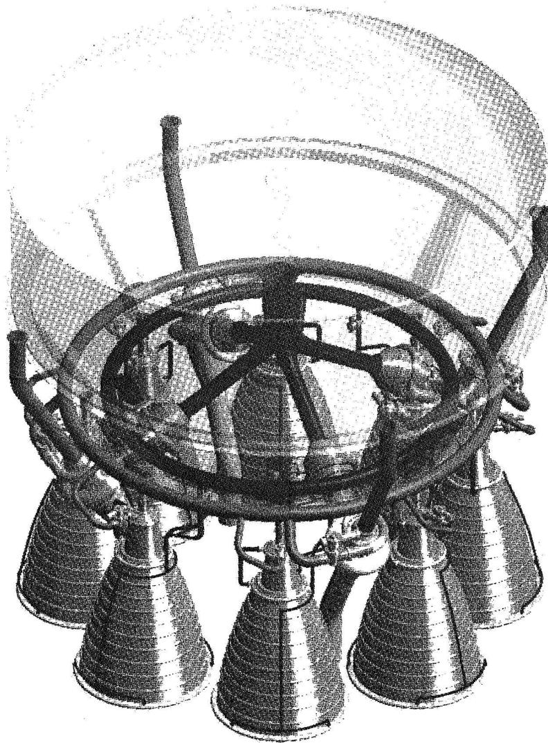
**Figure 2-1. Fully Integrated Booster Propulsion System**
