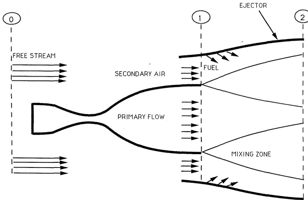
**Figure 2-3. Rocket Engine Air Augmented Afterburning Concept**
