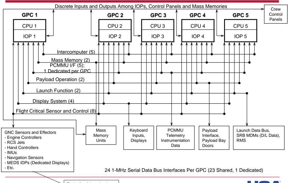
Session 8121 SHARE 2007, San Diego Typically triply redundant devices, connected to separate buses
