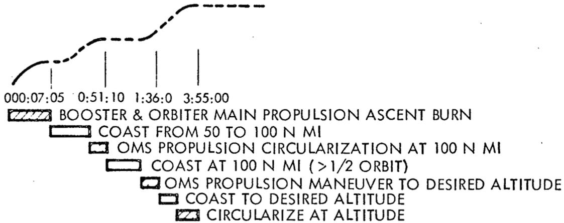
Figure 4-6. Sequence of Events, Core Module Delivery
