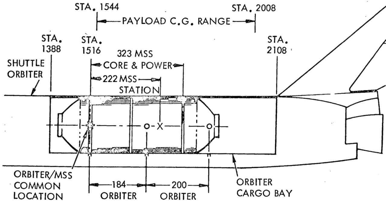
Figure 5-1. Variance Between Shuttle Cargo and MSS Module Support Locations
