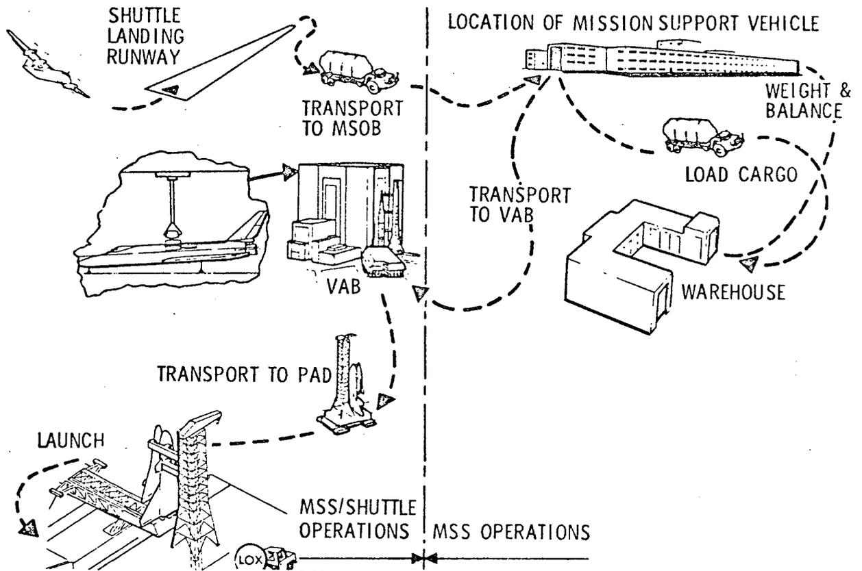
Figure 4-4. Typical MSS Module Flow at Launch Site
