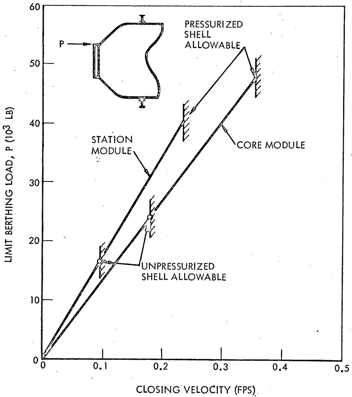
Figure 5-3. Berthing Load Versus Closing Velocity
