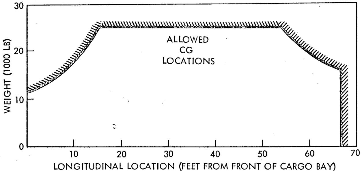
Figure 2-9. Payload Center-of-Gravity Envelope
