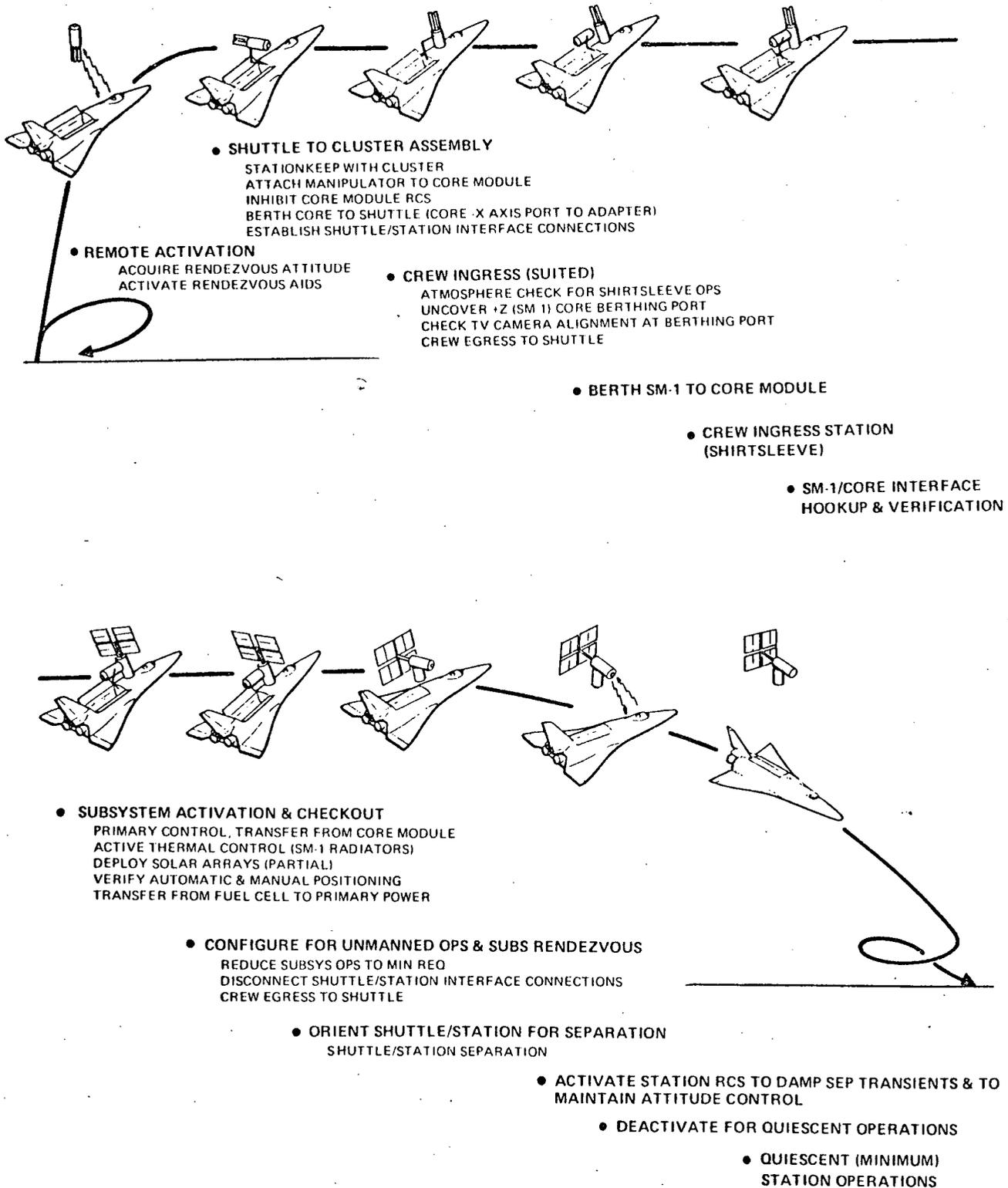
Figure 4-13. Typical Delivery Operations Sequence (SM-1 Delivery)
