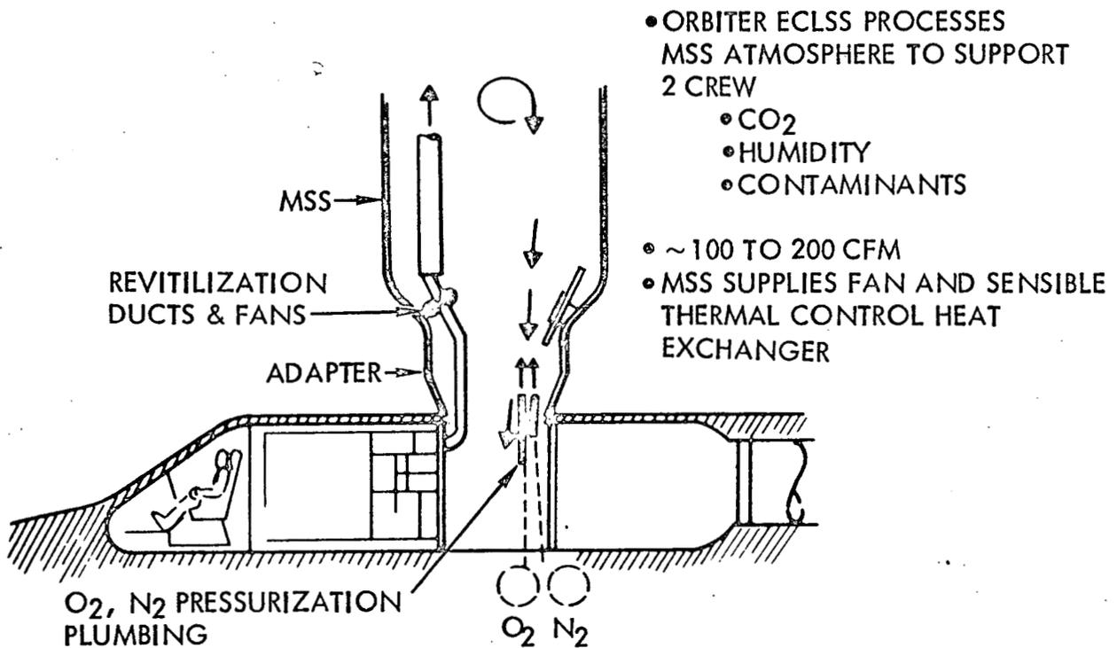
Figure 5-7. Atmosphere Revitalization of MSS
