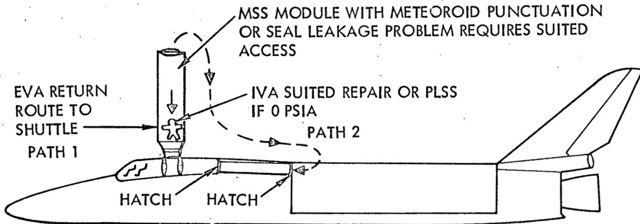
Figure 5-8. Orbiter-MSS EVA/IVA Provisions
