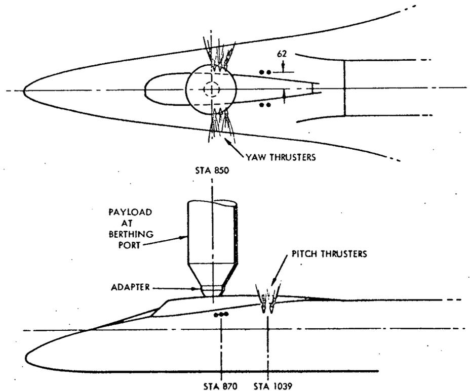
Figure 5-4. MSS-Orbiter ACPS Configuration
