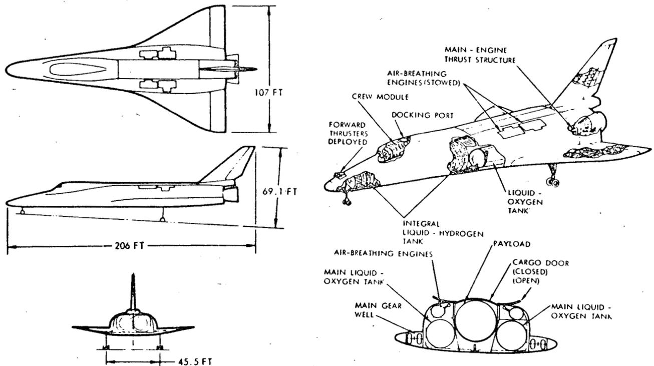
Figure 2-8. Orbiter Configuration
