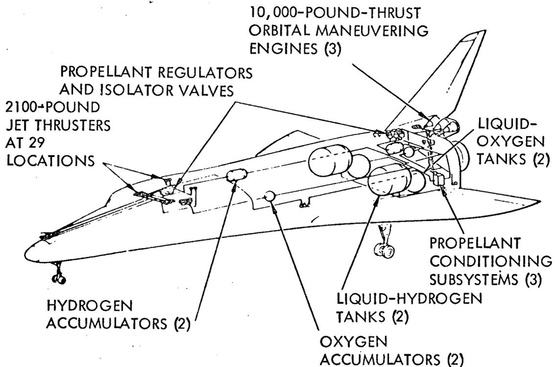
Figure 2-13. Auxiliary Propulsion System
