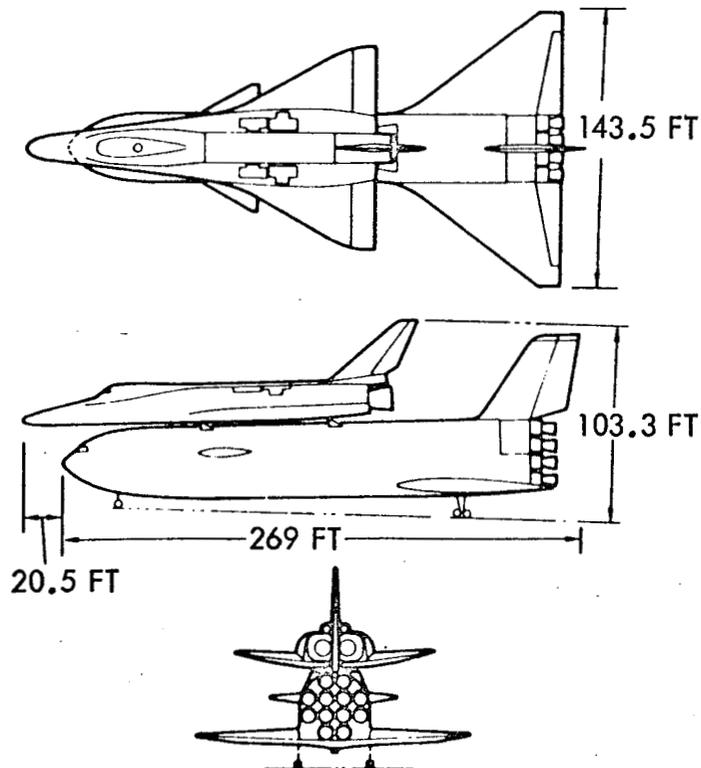
Figure 2-7. Mated Vehicle Configuration
