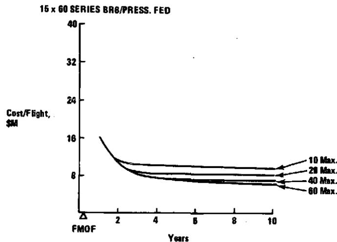
Figure 4-3 Operational Cost Sensitivity, 15 x 60 Series BRB/Pressure-fed
