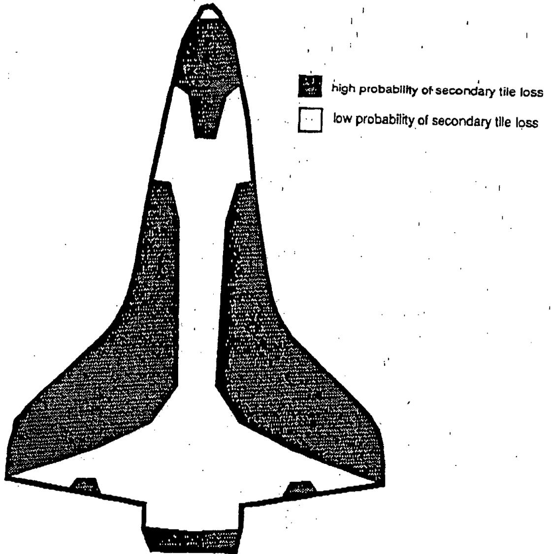
Figure 12: Partition of the orbiter's surface into two types of secondary tile loss zones (index: l)
