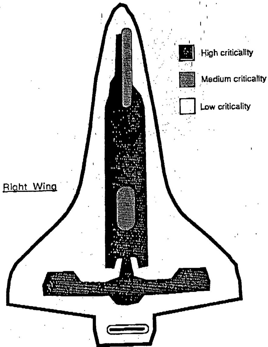
Figure 15: Partition of the orbiter's surface into three types of zones of functional criticality (index: j)
