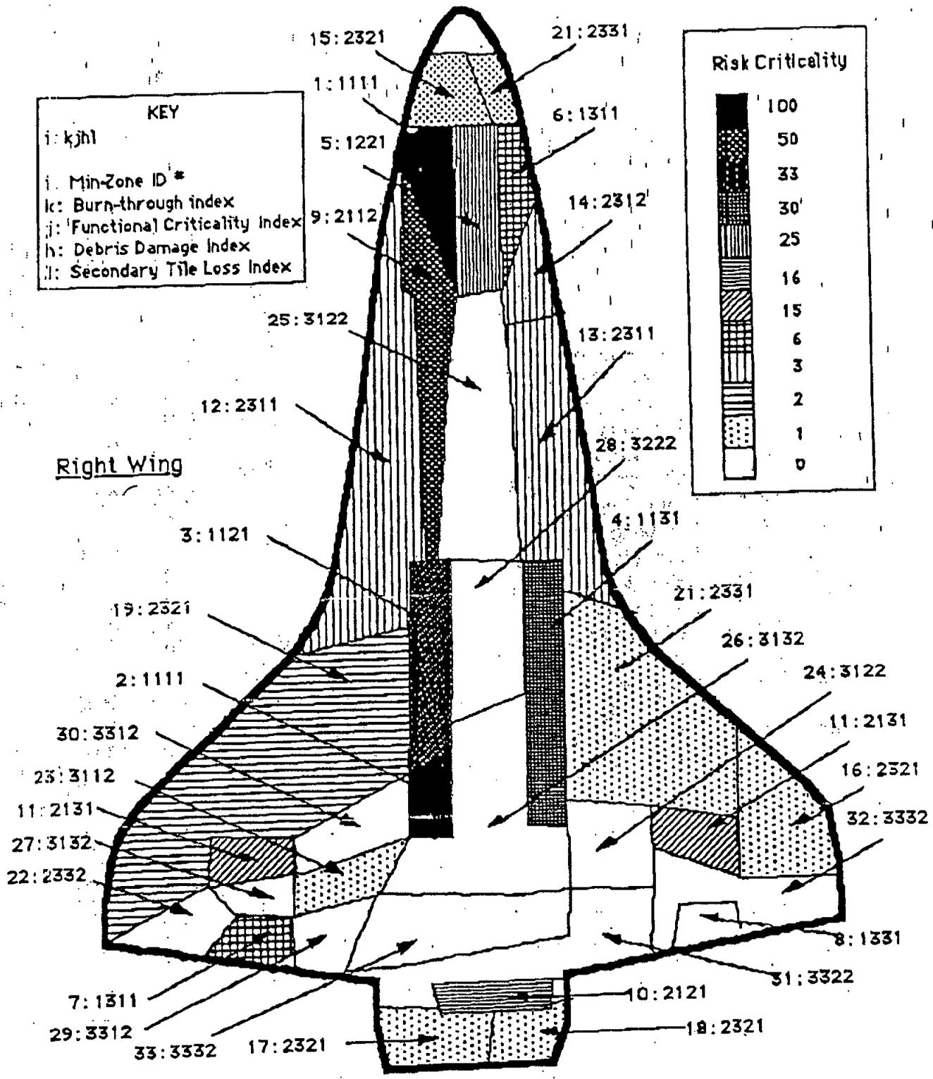
Figure 23: Partition of the orbiter's surface into 33 min-zones (index: i)
