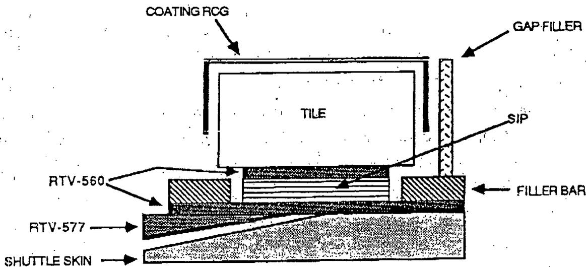
Note: Thickness exaggerated for clarity; Screed (RTV-577) only where needed
