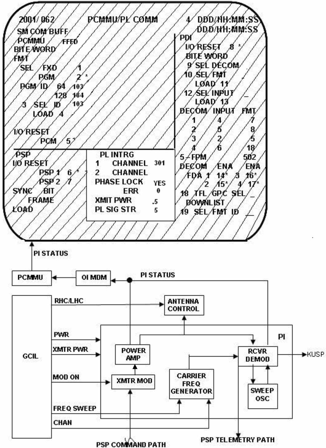
Figure 3-1. Payload interrogator
