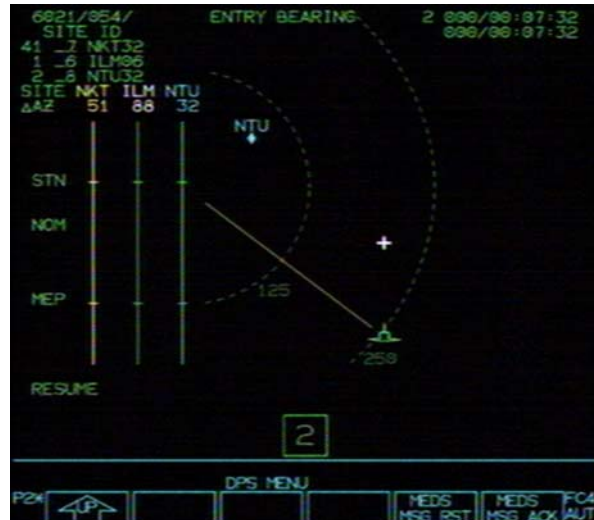
ECAL Entry to Cherry Point (NKT) with high ΔAz - MM602 pre Nz Hold
